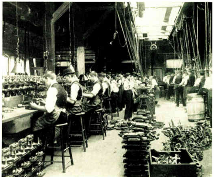
Fig. 8—The manufacturing and assembly department for the Shallenberger ampere-hour meter. This was located in the Garrison Alley Works (Pittsburgh) of the Westinghouse Company. Not until 1900 was manufacture moved to its location at Newark, N. J.
