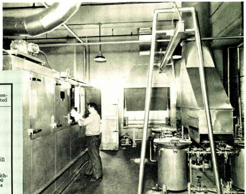
Fig. 2—For large-scale production of solventless-varnish treated transformers, a more elaborate array of tanks and ovens than usual is employed. The tanks at lower right are for evacuating and filling coils with liquid resin. Another tank is for coating the coils. The oven at left is large enough to provide the high baking temperature evenly throughout its interior with a large amount of air circulation.
