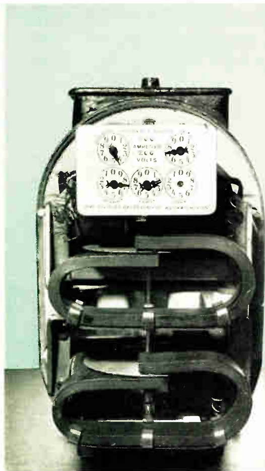
Fig. 9—The Davis-Conrad, two-disc, polyphase watt-hour meter. This was the first meter to measure correctly unbalanced polyphase loads, or to use separate discs for each element.
