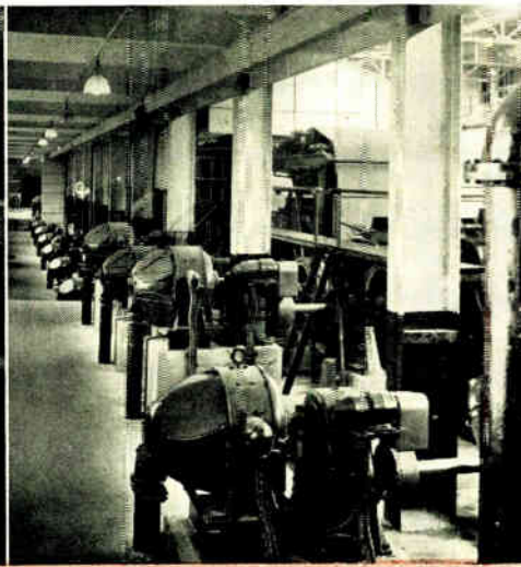
One of the largest Lifeline induction motors is the 600-hp, 3600-rpm unit (shown at left) driving a boiler feed pump. Each of these direct-current motors (right) drives a section of a papermaking machine. All machines must remain in step regardless of output speed.
