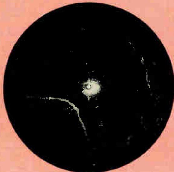
For close ranges (around the center spot) the use of the continuously variable sea-suppression control is extremely effective in disclosing objects that might otherwise be obscured by wave reflections. The two buoys and the ship in the right-hand view are hardly distinguishable in the left-hand view of the radar scope without using sea-suppressor control.
