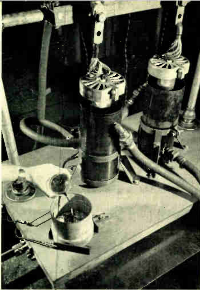
Fig. 2—A cutaway portion of part of the ignitron was left open so that engineers could actually observe the movement of the mercury. Here mercury is being placed in the cutaway tube, in preparation for tests.
