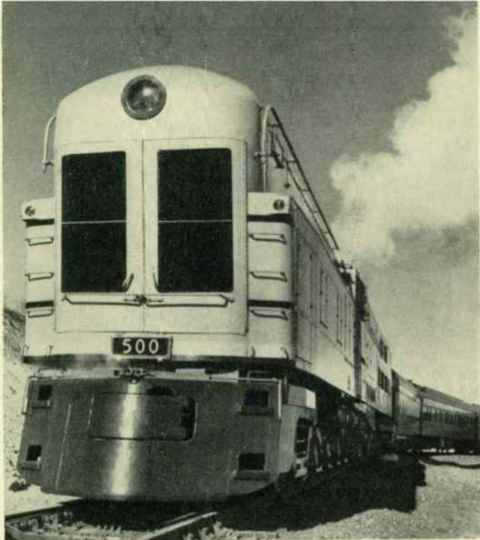
One of three steam-turbine, electric-drive locomotives in high-speed passenger service on the Chesapeake & Ohio Railway.
