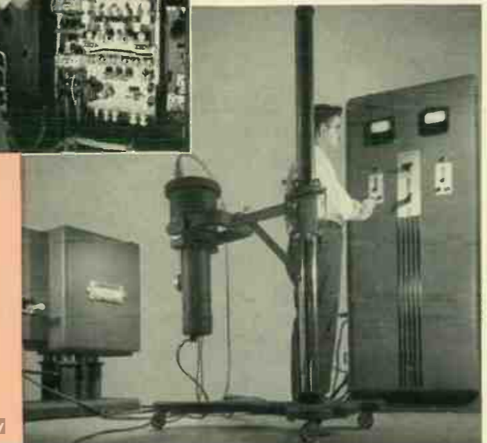
The high-speed x-ray motion picture device has gone from the seeming disarray of apparatus that characterizes many research setups to neat, compact cabinets, operated by pushbuttons. Film speeds are 50, 100, or 150 frames per second; exposures, each 10 micro-seconds.
