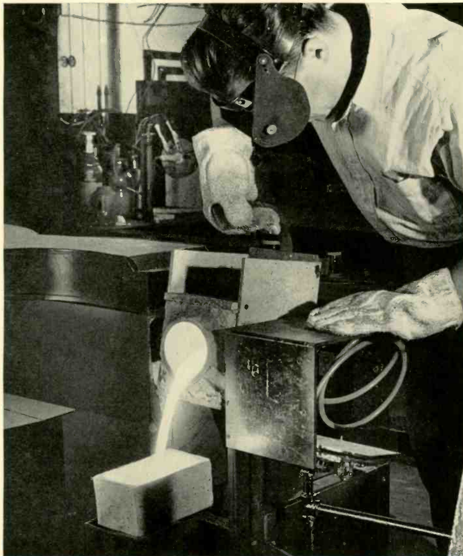
A carefully prepared "recipe" of metals is poured from a high-frequency furnace to form an ingot of Hiperco, a new magnetic alloy with extremely high saturation.
