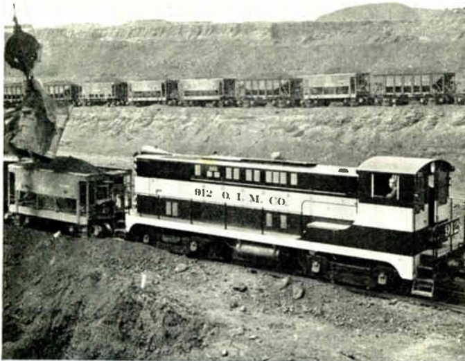
On the Mesabi, much of the ore is scooped up by electric shovels and loaded directly into cars for haulage to Duluth.
