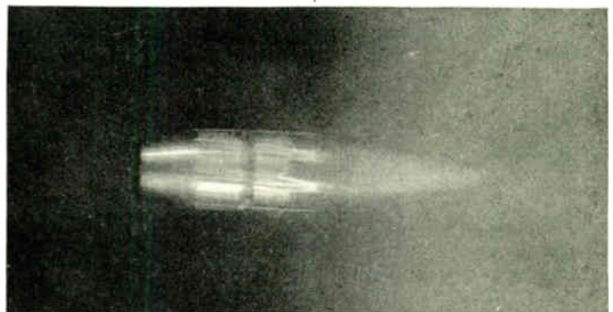
Fig. 11—To take this light-picture of a bullet in flight the x-ray tube was removed and the surge generator discharged across a gap to give an intense but extremely brief light.
