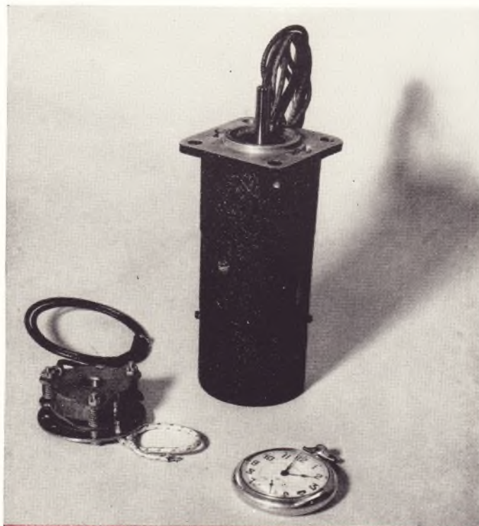
A quick-acting brake lies beside a d-c motor for airplane service. The brake fits inside the motor housing.
