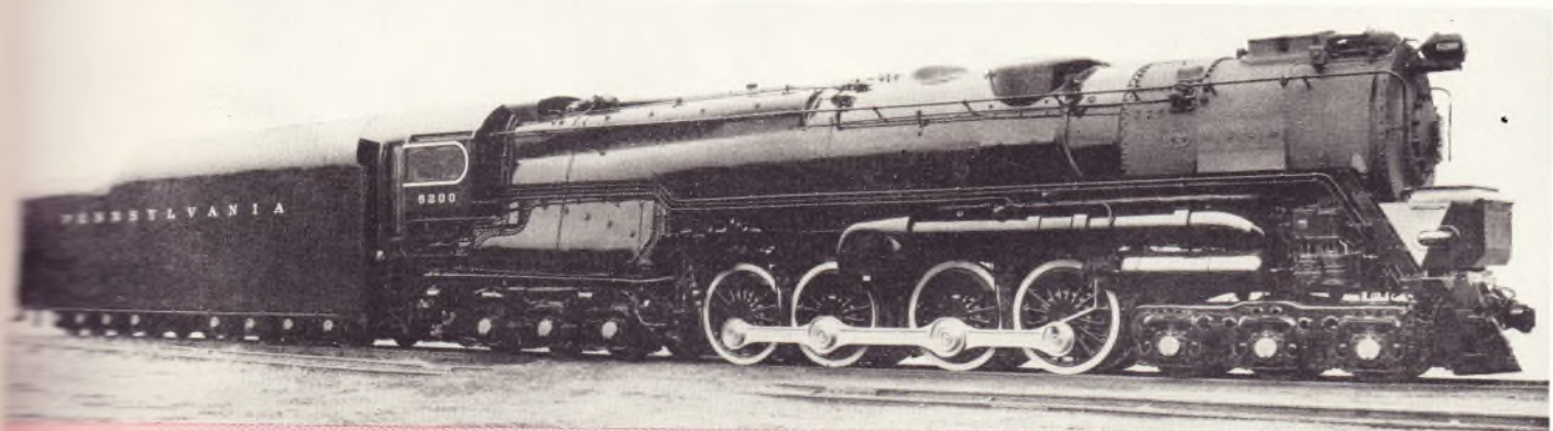
The first locomotive driven by a geared steam turbine, built in this country, has successfully completed its initial trials.
