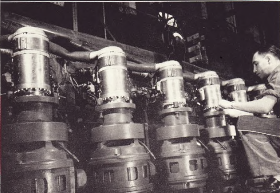
(Top view) Gyroscopes, with their mirror-polished inertia wheels, are machines of extremely accurate balance and great precision. (Center view) Here is a gunner's eye view of a target as seen through a gunsight with its reticule lighted by a greatly improved gunsight lamp. (Bottom view) Generators are given run-in tests of several hours, in addition to various electrical tests. These generators, mounted atop the driving motors, are the famous P-1, in service on all fighting fronts.
