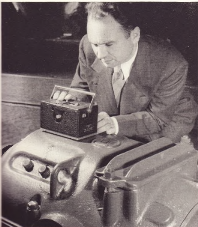
The portable vibration recorder mechanically amplifies the vibration and traces it with a record of time on a ribbon.
