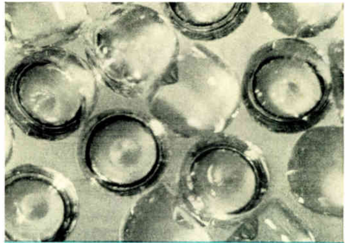
Glass instrument bearings as seen under a microscope. These "jewels" are so inspected to check depth and angle of the cavity.
