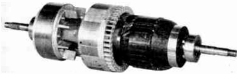
Motor-alternator shaft assembly; generator rotor with cooling fan in center
