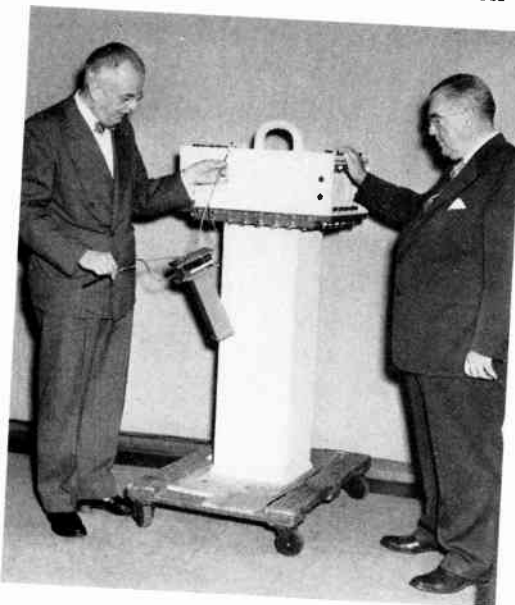
Vice-President in charge of Development and Research H. P. Corwith (right), and Transmission Research Engineer F. B. Bramhall (left), examine 1100-pound submerged cable repeater as they view a scale model showing how submarine conductor enters and leaves the unit
