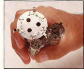
Fig. 2: Sizes of CRT's have changed dramatically over the years from the old Delta gun style to today's newest in-line. The smaller in-line gun produces much better convergence.
