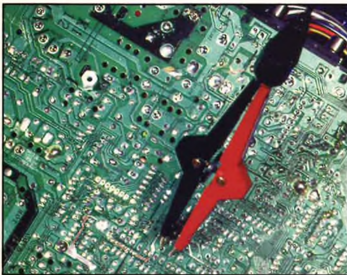
Fig. 3: Testing components in-circuit eliminates wasted time.
