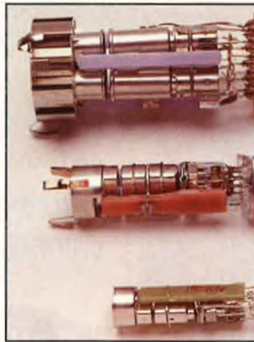
Fig. 1: Today's electronic guns have gotten smaller and are capable of producing better quality pictures.
