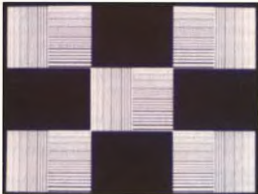
Fig. 6: The blurred 1-pixel vertical lines indicate poor horizontal resolution.
