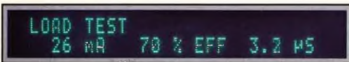
Fig. 3: The load tests showed normal readings for a monitor operating at 68 kHz.
