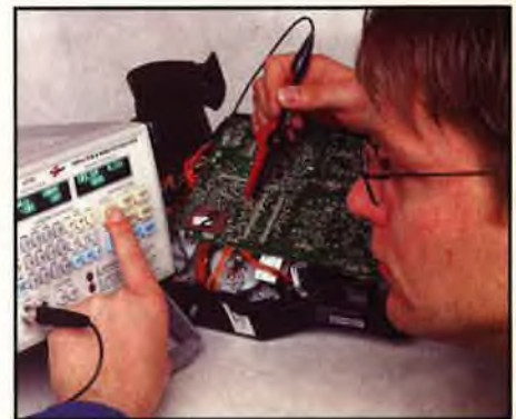
Fig. 1: The in-circuit test probe allows convenient and quick connection to both component terminals.
