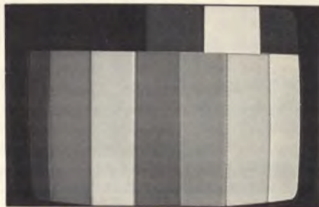
Fig. 11: The white bar of the split field pattern is on the same line as the "-I" and "Q" bars, causing an overlap when viewed on an oscilloscope.
