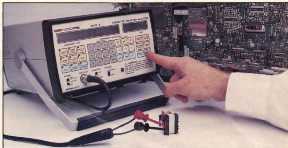
Fig. 8: The LC77 will identify shorted turns in the switching transformer. A shorted turn will destroy the switching transistor.
