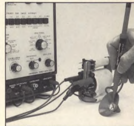
Fig. 4: The same connections to the primary are used for the driving test as were used for the ringing test.
