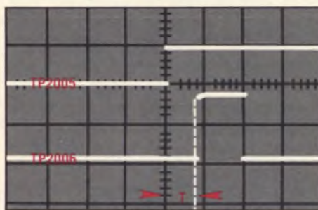
Fig. 6: The instructions call for careful CRT graticule counting to set the Tracking Fix adjustment.
