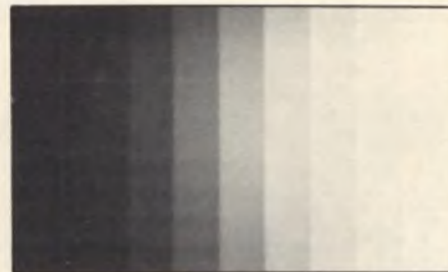
Fig. 12: The VA62 10-Bar Staircase video pattern (top) provides samples of ten different video levels (bottom), producing different VCR modulation frequencies.
