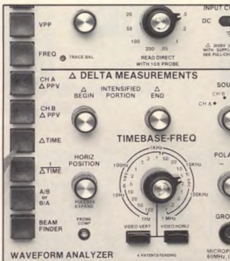
Fig. 7: Pressing the Delta time button activates the Delta Begin and Delta End controls which position an intensified bar on the CRT waveform.
