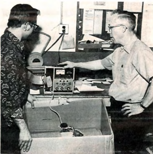
Stan Oestreich, left, Sencore engineering technician looks on as Gary Akins of Warren Radio explains how they use the CR161 Auto Tracker to check each warranty picture tube returned.
