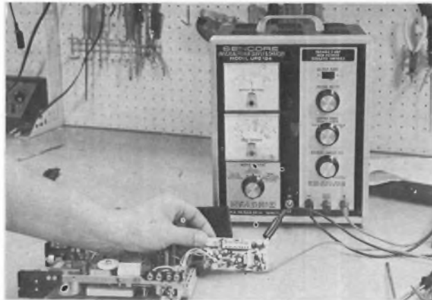
Recorder servicing is easy when board can be removed and powered with UPS164.
