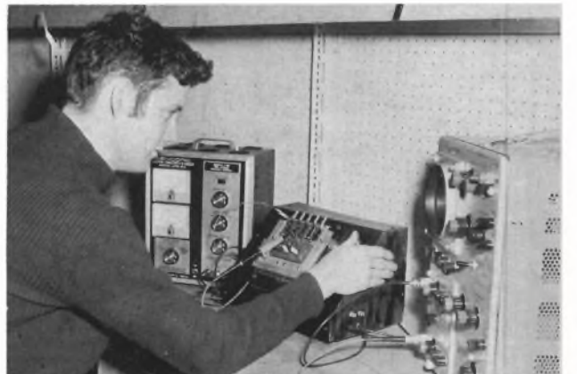
UPS164 powers production line test fixture in large electronics manufacturer.
