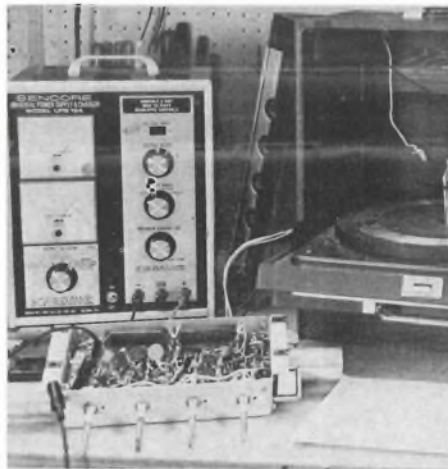
Phono servicing is greatly simplified when you have a UPS164 to provide operating power.
