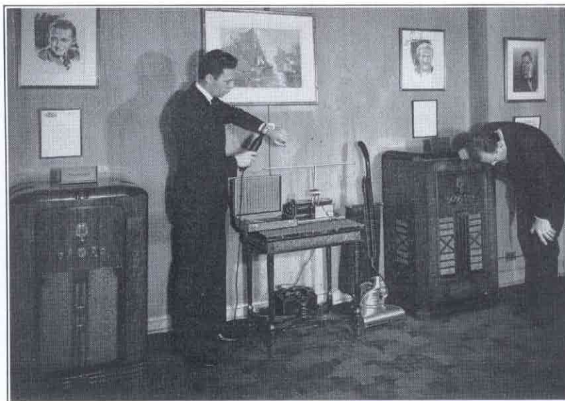
View in One of Studios Showing the Violet Ray Machine, Vacuum Cleaner and Spark Coil Used to Create Electrical Interference and Prove How Scott Supershield Antenna Coupling System Eliminates 99% of It.
