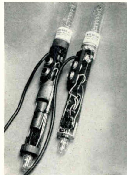
Figure 1. Two types of photo flash guns using SYLVANIA tubes. The SYLVANIA Type OA5 trigger tube can be seen on the lower end.
