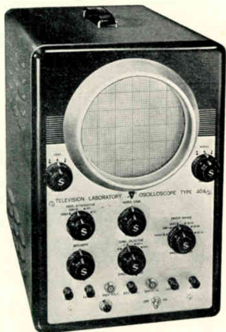
Figure 1. Sylvania Model 404 Laboratory Oscilloscope. This instrument is particularly suitable for use in observance—without distortion—the sawtooth, square-wave, and other pulses found in television equipment.
