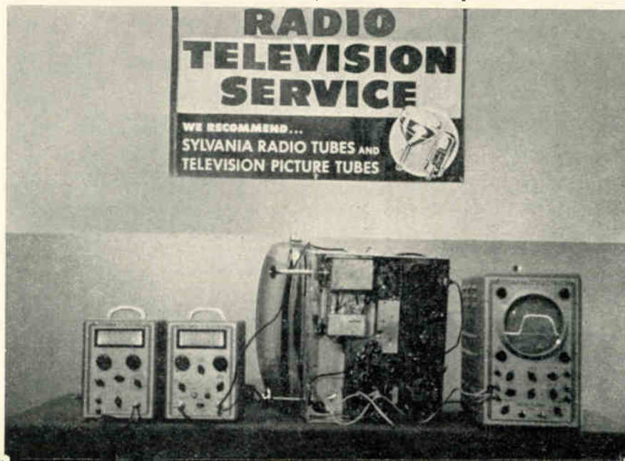
Figure 1. TV alignment set up. From left to right is the Sylvania 500 sweep generator, 501 marker generator, Sylvania TV set and Sylvania 400 oscilloscope.
