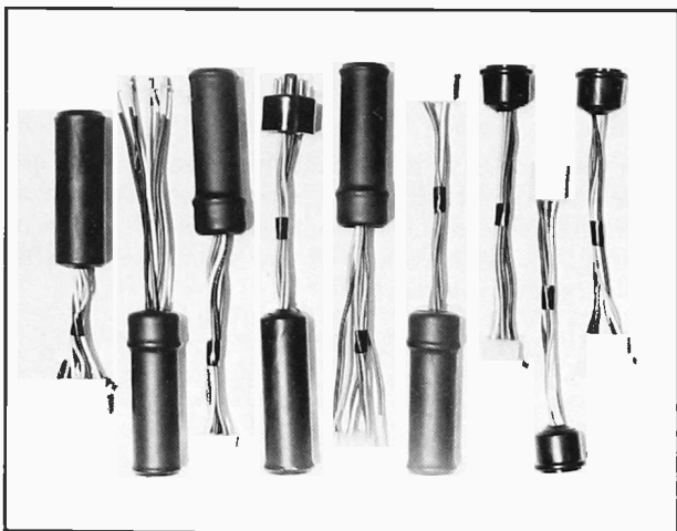
Representative Adapter/Extension Kits for Chek-A-Color Test Jig. Upper photo shows universal kit—used with most chassis—while lower photo is that required for the chassis of one typical receiver make.
