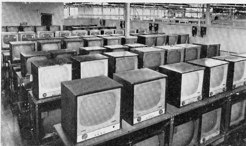
FIGURE 5—TV LIFE TEST. Tubes are life tested in TV receivers representing many different makes and models, for a period approximately equivalent to one year of set operation.
