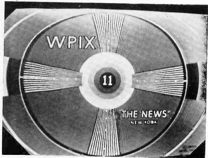
CONDITION—Poor vertical linearity. CAUSE—(A) Misadjustment of the vertical linearity control, or (B) The vertical deflection tube should be checked for defective operation, and if defective, it should be replaced with a new tube.
