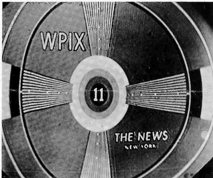
CONDITION—Pattern is non-linear in the horizontal direction. CAUSE—(A) Horizontal drive control or linearity coil out of adjustment. (B) The damper tube is defective.
