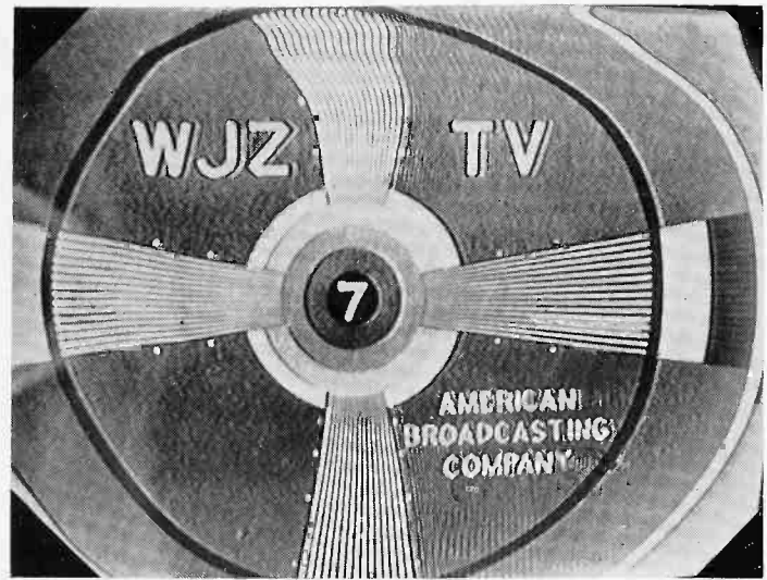
CONDITION—On verge of losing horizontal synchronization. CAUSE—(A) Misadjustment of hold control or phase control. (B) Defective horizontal sync amplifier tube or component.
