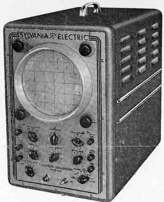
FIG. 1—The circuit features of the Type 400 Television Oscilloscope which make it a good television service instrument also make it a good instrument for general purpose laboratory and industrial use.
