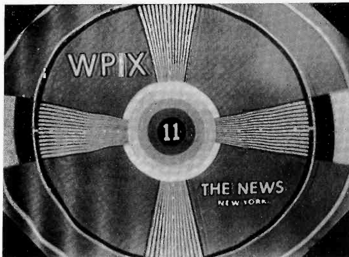
CONDITION—Several bright bars at left side of the screen cause the pattern to appear wrinkled. CAUSE—Oscillation in the yoke due to an open or wrong value of condenser across the top half of the horizontal winding of the yoke.
