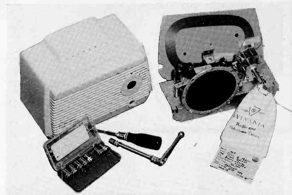
Use of the new Sylvania parts bag is illustrated above. Knobs, chassis screws, and other small parts can be stored in the bag while the set is undergoing repair. Parts bag also has attached job ticket for record keeping and customer receipt.
