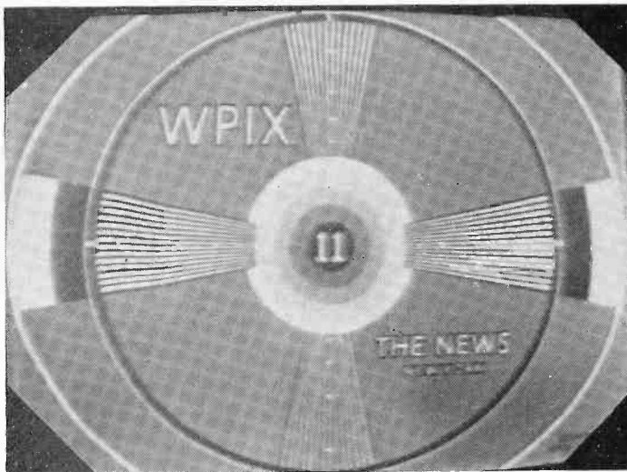
CONDITION:—Poor resolution of vertical wedges and the retrace lines are visible (low gain). CAUSE:—Load resistance of the video amplifier is increased due to the opening of a plate peaking coil which was shunted by a resistor.
