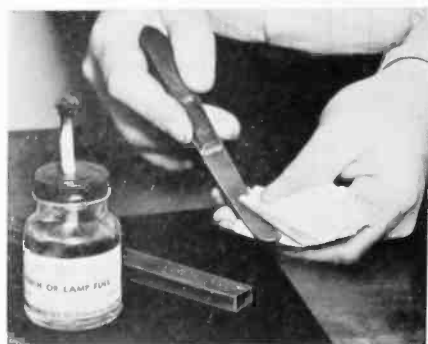
1. After heating spatula wipe clean with cloth to remove carbon deposit.
