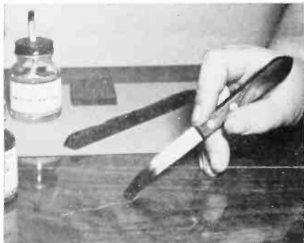
3. Spread shellac on spatula into scratch or cut and allow to thoroughly harden.
