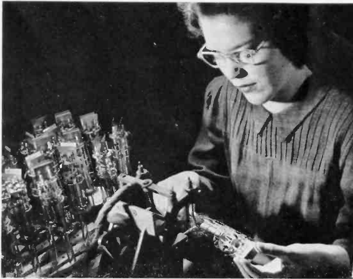
FIGURE 4. A step in assembling an electrostatic type gun.
