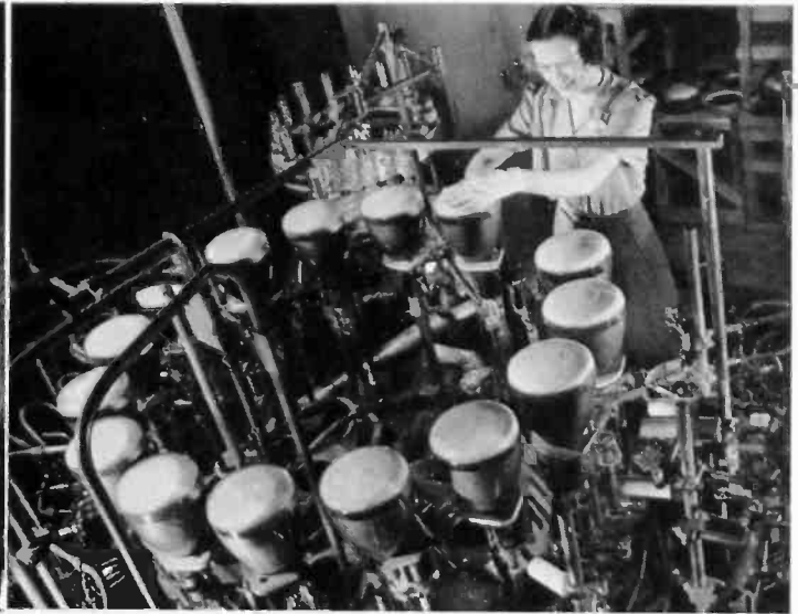
FIGURE 5. The mount is sealed into the bulb in this machine.
