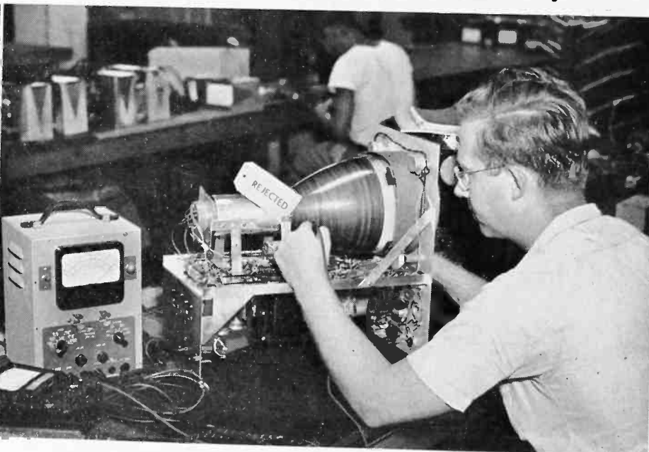
Instruments which reveal inaccuracies in final test are returned to engineers who check every part and connection for quality. Note—Polymeter used for testing.
