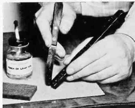
2. Melt shellac stick onto spatula by holding it against heated spatula.
