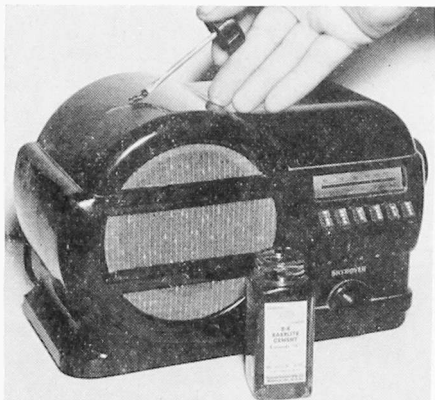
Use plastic cement in making repairs on moulded plastic cabinets.
