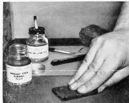
4. Smooth shellac with felt pad containing shellac stick rubbing fluid.
