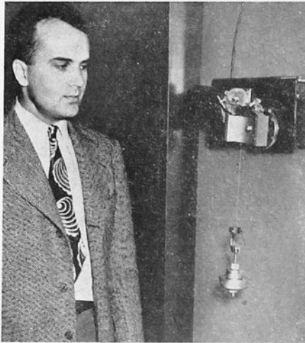
D. W. White, a member of the laboratory staff, is engaged in the study of the fundamental properties of tungsten wire. He was primarily responsible for establishment of the operating principles and the development of the new fissure tester shown at right.
