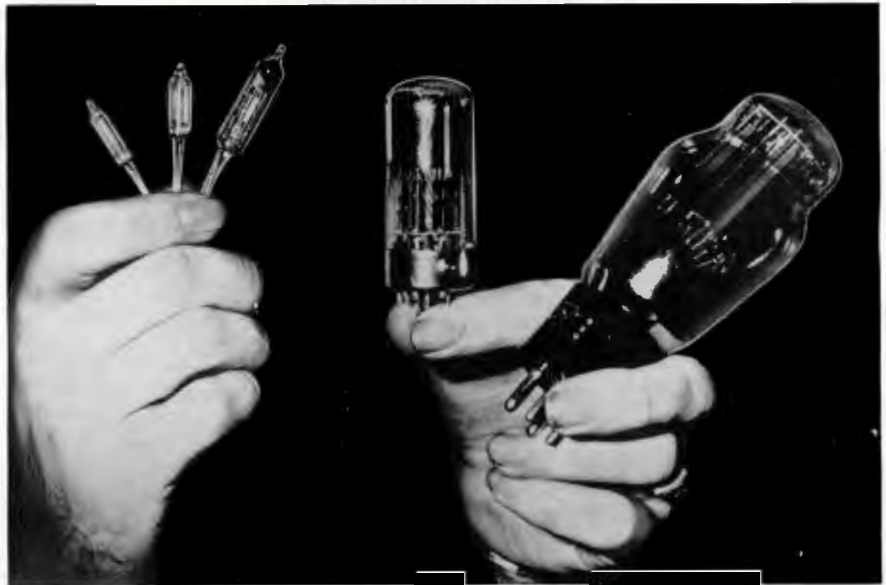
Right to left: A conventional Sylvania tube of 10 years ago, a current lock-in tube, the proximity fuze tube, the T-2, and T-1.
