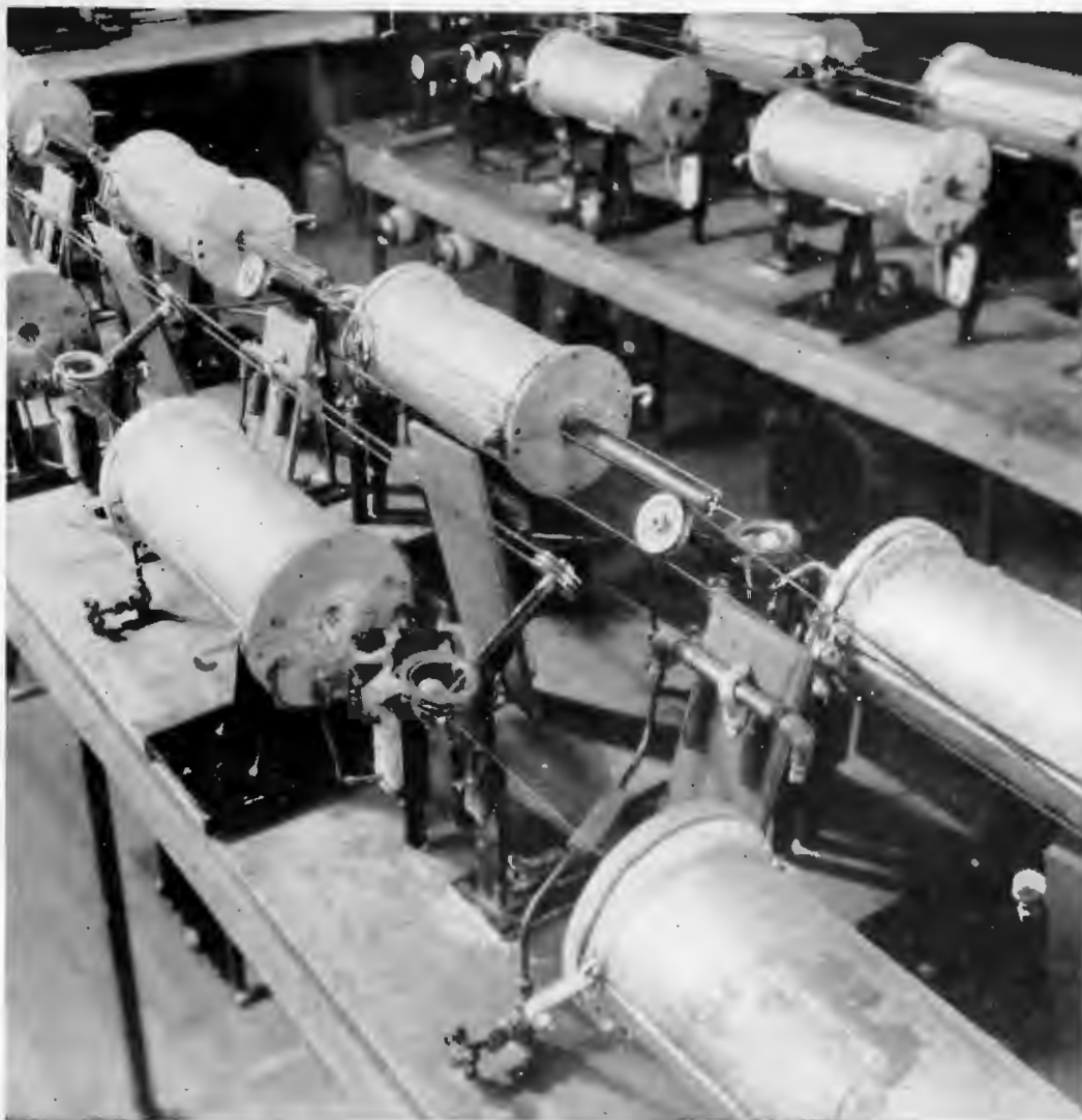
WIRE COATING MACHINE. This machine is used for coating heater wire. The wire is drawn through the mixture of insulating oxides and the coating is baked on in passing through the electric oven.
