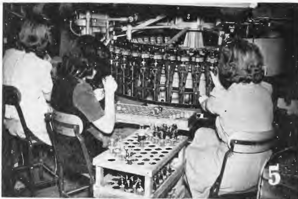
5. This machine keeps the bulb and base in perfect alignment while the cement holding them together is baked on. The operators of this machine also cut off and solder the wires as the tubes are taken off.
