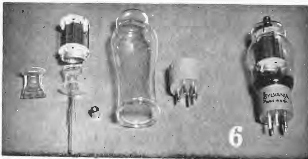
6. From left to right this shows a flare; a complete mount, top cap, bulb, base and a completed Sylvania type 807 tube.
