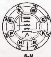
Sylvania Type 12B7 Triple Grid Amplifier
