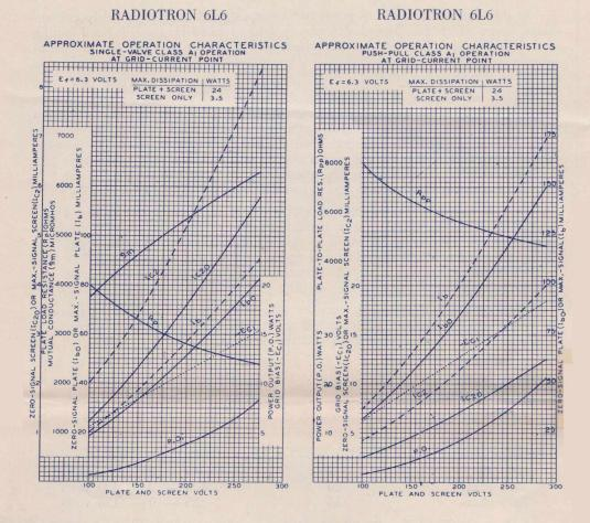
The total plate and screen dissipation of the 6L6 should not exceed 24 watts and that of the screen itself should not exceed 3.5 watts. The screen dissipation increases with power output because of rectification in the screen circuit; plate dissipation decreases with increasing power output. Hence the maximum screen dissipation value should not be exceeded with full signal applied and the maximum plate and screen dissipation value should not be exceeded when no signal is applied.
