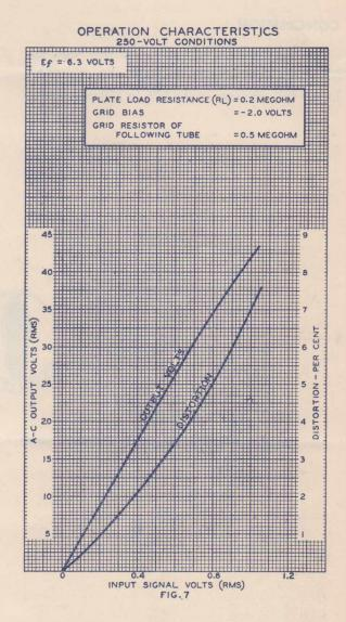
gain and distortion requirements. For most radio receiver applications, a bias of -2.0 volts and a plate load resistance ( $R_L$ ) of 0.2 megohim are suitable.
