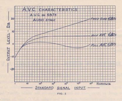
use of infinitely high screen dropping resistance. A compromise has therefore been adopted (Fig. 1) which incorporates a potential divider for screen voltage supply. The value of the resistor from In Fig. 2 the working path with the specified potential divider is shown as a dash line and it will be seen that the characteristic is substantially linear from -2 volts to -8 volts on the control grid.
