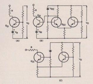
Fig.3 - Three typical dc amplifier elements.
