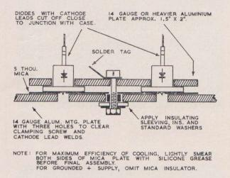
Method of arranging the two silicon diodes with a common positive connection, and heat sinking them.
