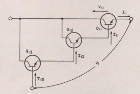
Fig. 2 - Series regulating element consisting of two or more transistors in common-collector configuration.
