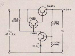
Fig.6 - Complete circuit for transistorized series voltage regulator.
