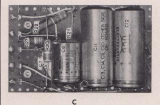
Component layouts in (A) driver and predriver section, (B) output stages, and (C) power supply components.
