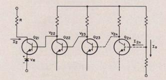
Fig.11 - Typical cascaded dc amplifier element.
