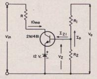
Fig.5 - Amplifier element for series voltage regulator.
