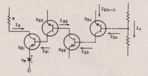
Fig. 12 - Tandem connection of transistors used to produce high gain and a high degree of temperature stability.
