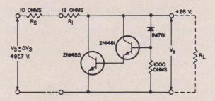
Fig. 9 - Complete circuit for transistorized shunt voltage regulator.
