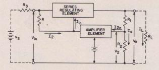
Fig.1 - Typical transistorized series voltage regulator.
