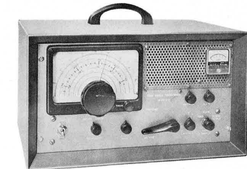
FIGURE 1: W2OKO's two-meter transceiver features large dial with vernier for easy tuning. All operating controls of the unit are located on the front panel.
