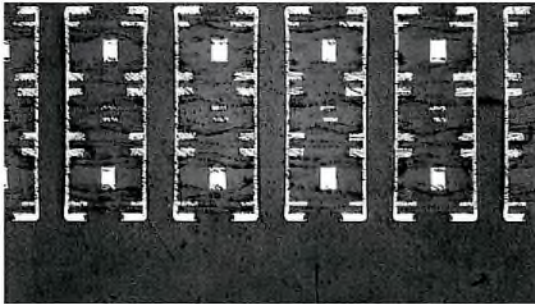
A row of 5 via holes on a pitch of 1.27 mm, drilled 0.4 mm in a multilayer board 2.8 mm thick. Two CIC planes of 0.25 mm, and 10 coppers layers can also be seen
