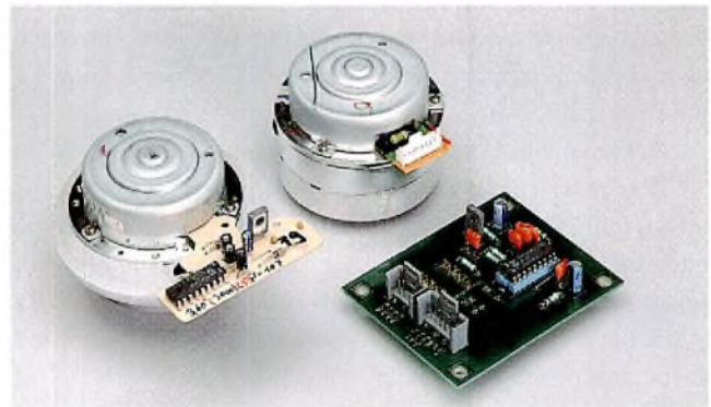
Fig.8 An application evaluation board using the TDA5140A to drive a VCR scanner head motor
