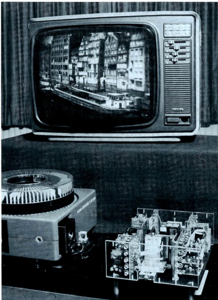
Fig.11 The TV screen displays the slide projected onto the laboratory model P 2 CCD scanner in the foreground.
