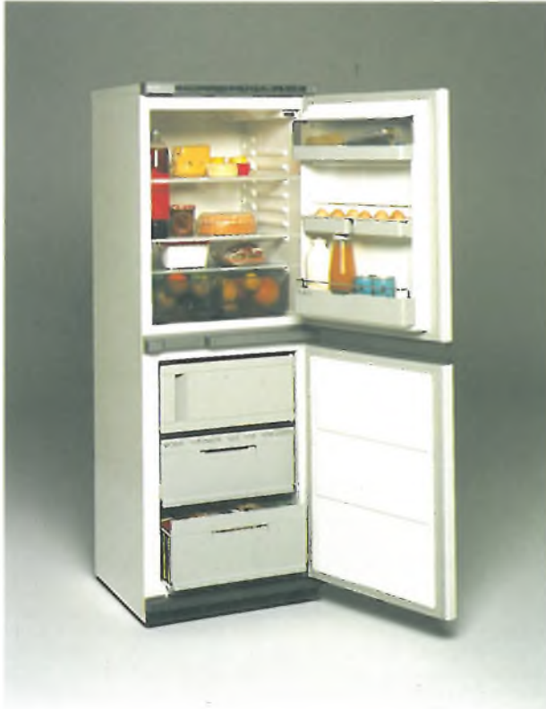
Fig. 4. The Philips ARG 197 refrigerator-freezer. The refrigerator is at the top, the freezer below. The appliance has only one compressor unit and has electronic temperature control, with a temperature sensor in both the refrigerator and freezer compartments. The control circuit operates a valve that divides the refrigerant between the two evaporators in the two compartments.
