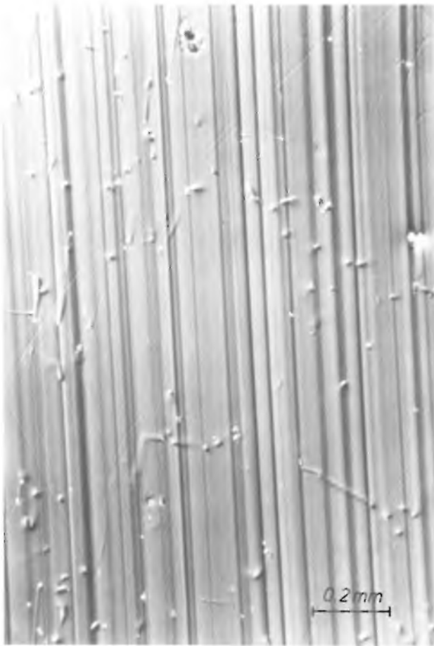
Fig. 13. Photomicrograph (interference contrast) of n-GaAs after photo-etching with an \text{H}_2\text{O}_2/\text{H}_2\text{SO}_4 solution for revealing crystal defects [8] .
