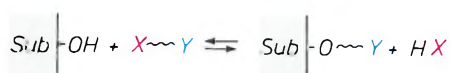
Fig. 1. Diagram illustrating the chemical modification of surfaces. A substrate surface Sub , on which reactive groups are present (a hydroxyl group is shown here), is allowed to react with organic molecules possessing two functional groups. One functional group, X (red), reacts with a hydroxyl group, the other, Y (blue), provides the surface with the required new property.
