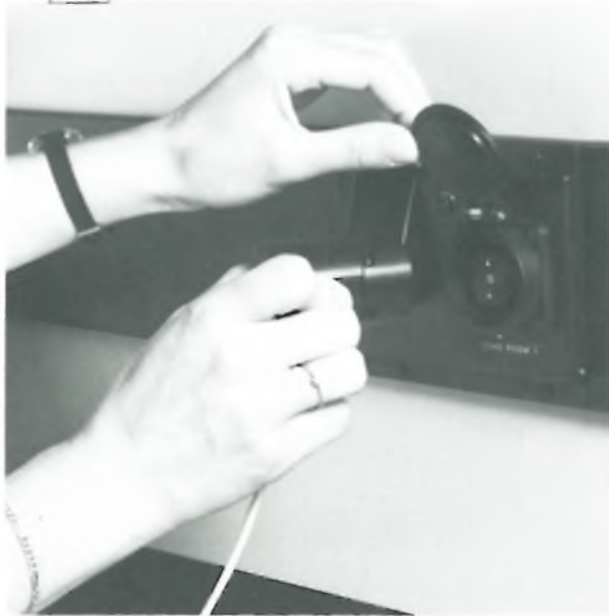
Fig. 14. Wall socket and plug for the PHILAN meander ring. This provides a reliable and easily detachable double optical and double electrical connection (see fig. 12a) [12] .
