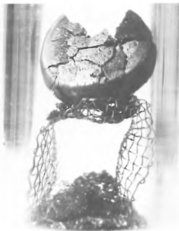
Fig. 6. If \text{LaNi}_5 is made to absorb and desorb hydrogen repeatedly, it gradually disintegrates into small fragments, seen here in a small heap under the piece of metal gauze acting as a sieve. (This is the effect of a single absorption of hydrogen by an \text{LaNi}_5 casting.)
