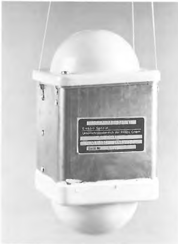
Fig. 10. a ) Principle of locating the position of a radiosonde by means of a transponder, a combination of a transmitter and a receiver. The transponder, which is suspended from the balloon of the radiosonde, responds to a signal transmitted by a parabolic antenna on the ground. The position of the radiosonde can be determined from the angles at which the ground station receives a signal from the transponder, and from the time that elapses between the transmission and reception of the signal. b ) The transponder, complete with antennas, which are located underneath the top and bottom shielding caps. The transmitted power is 200 mW and is sufficient for a range of 50 km. The transponder contains a microwave oscillator with dielectric resonator and is a product of the Philips GmbH supply centre Systeme und Sondertechnik in Bremen.
