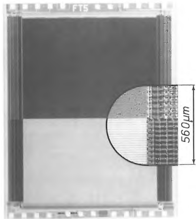
Fig. 8. The accordion imager. The storage section (the light region) is smaller than the image section (the dark region). The storage section is shielded from light by an aluminium layer. The n-channels are vertical, the CCD electrodes horizontal. On the left and right are the shift registers, which generate the voltages on the CCD electrodes. Insert: enlarged view of the transition from image section to storage section.
