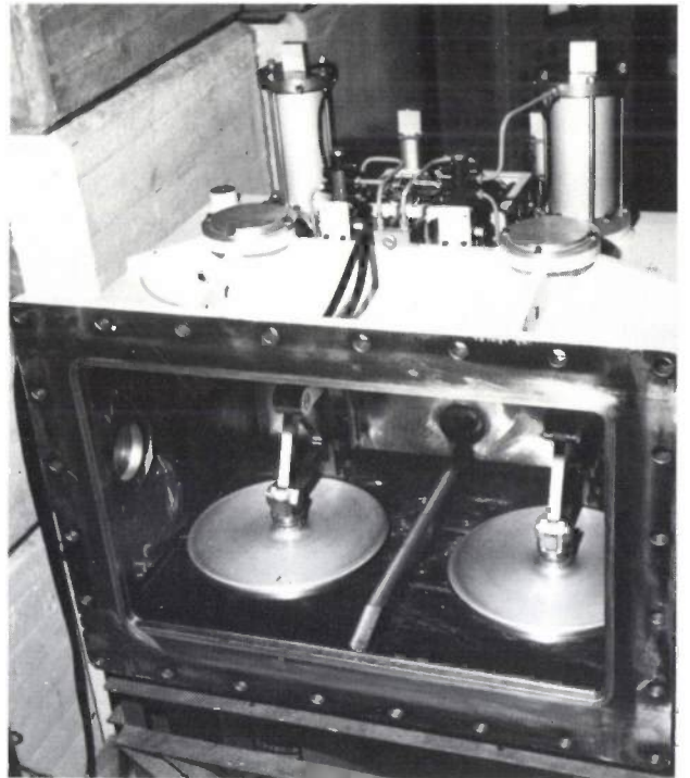
Fig. 3. Some examples of vacuum valves with orifice diameters between 8 and 35 cm. One of the features of these valves was that they could be operated either by hand or by compressed air.
