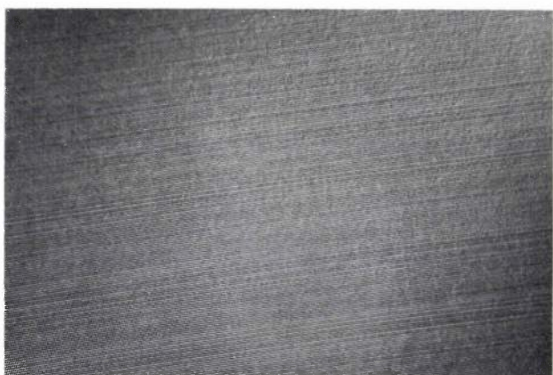
Fig. 5. Photographs of aluminium surfaces that have been turned with a diamond-tipped tool (magnification 35×). Above : surface of engineering-grade aluminium. Below : surface of 35 µm electro-deposited aluminium on engineering-grade aluminium. The quality of this surface is clearly much better.
