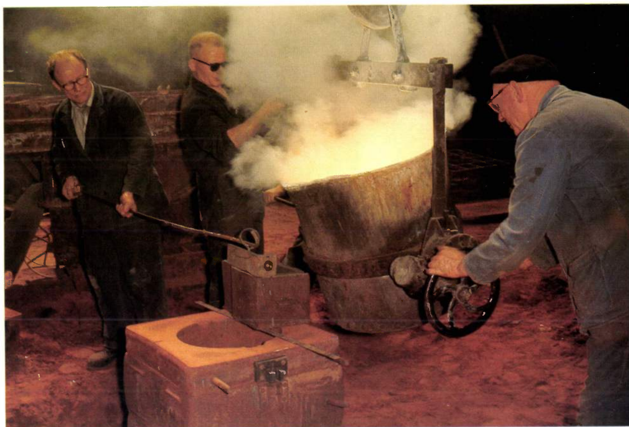
Casting one of the inner copper hemispheres for the BOL nuclear measurement project.
