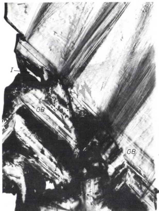
Fig. 13. Transverse X-ray topograph (above) of a (100) slice sawn from the grown tetragonal cap of a DKDP crystal, and schematic representation of the cap formation (right). Dislocation lines are generated if the (011) and the (0 \bar{1} 1) sectors of the same pyramid have different lattice constants (arrow 1), or if the two merging (011) sectors of the adjacent pyramids A and B are at an angle to each other (arrow 2). The topograph also shows the inclusions I and the growth bands GB mentioned earlier.
