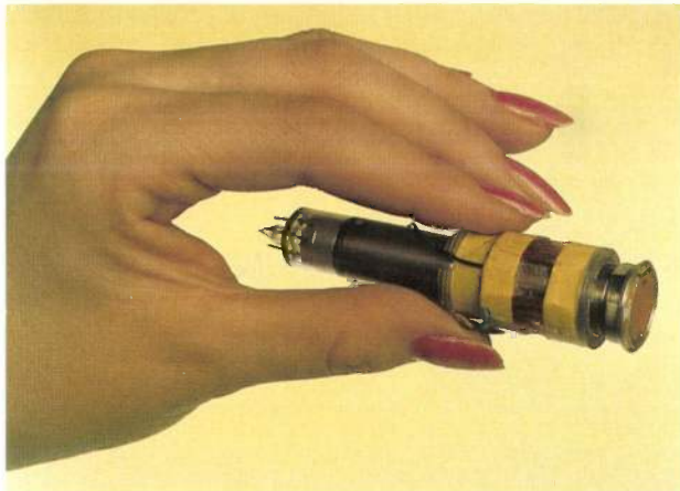
Fig. 14. Photograph of an experimental Plumbicon tube in a coil unit, made with the new technology on the basis of the new electron-optical design.
