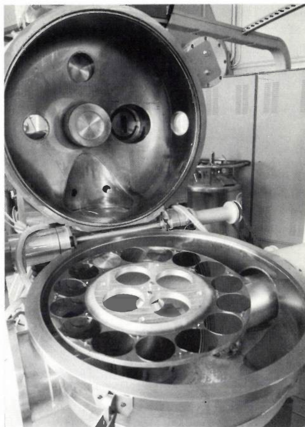
Fig. 4. Target chamber (opened) of a system for high beam currents. The specimens are mounted on a disc, which rotates during the bombardment; the disc is then in the vertical position.
