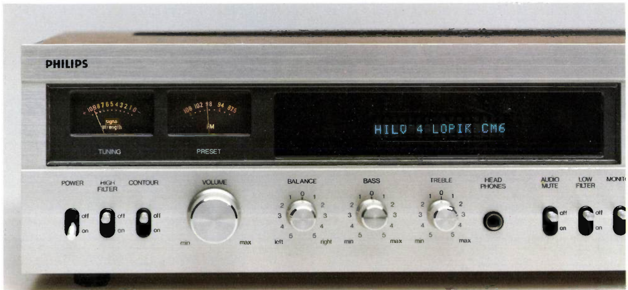
Fig. 1. The 794 receiver, with a display for SPI messages. The display indicates that the receiver is tuned to the programme Hilversum 4, transmitted by the station at Lopik and that at that moment the particular programme item being transmitted is CM6 (classical music No. 6). The display is a vacuum fluorescent display (VFD).
