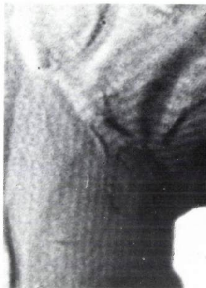
Fig. 14. X-ray topograph of a (001) slice of a DKDP crystal sawn off close to the seed crystal before the final growth habit has been attained. Observe the continuity of the 'Pendellösung' fringes at the boundary between the pyramidal sectors. Fringe deformations are due to thickness variations.
