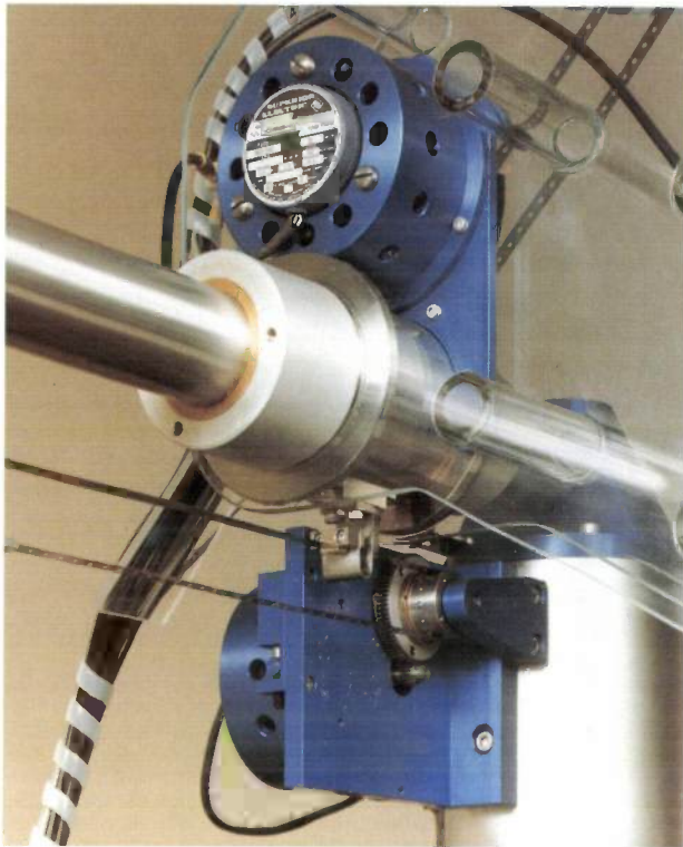
Fig. 4. Part of the equipment. The air bearing for the r -displacements can clearly be seen. Below it is the stepping motor which produces these movements. Above it can be seen the stepping motor for the z -displacements.
