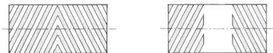
Fig. 7. Herringbone pattern for a completely grooved bearing surface ( left ) and for a partially grooved bearing surface ( right ) in a spiral-groove journal bearing. The two groove patterns are symmetrical: the two sections of the herringbone that pump lubricant to the centre are of the same length. When grease is used as the lubricant an asymmetrical pattern is preferred.
