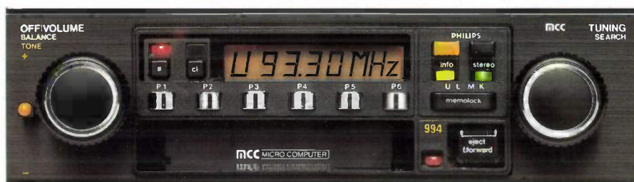
Fig. 2. The MCC (microcomputer-controlled) car radio has a memory in which ten station frequencies can be stored for each of six different programmes ( P1 to P6 ). The receiver automatically searches for the frequency with the strongest signal.
