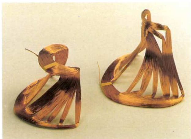
Fig. 5. Saddle coil for the 20AX ( left ) and 30AX ( right ) systems. For the 20AX the coils have a 'flange' at the neck side, which complicates the structure of the deflection unit, since neither the plastic carrier nor the yoke can be made in one piece. There are no flanges in the 30AX system.
