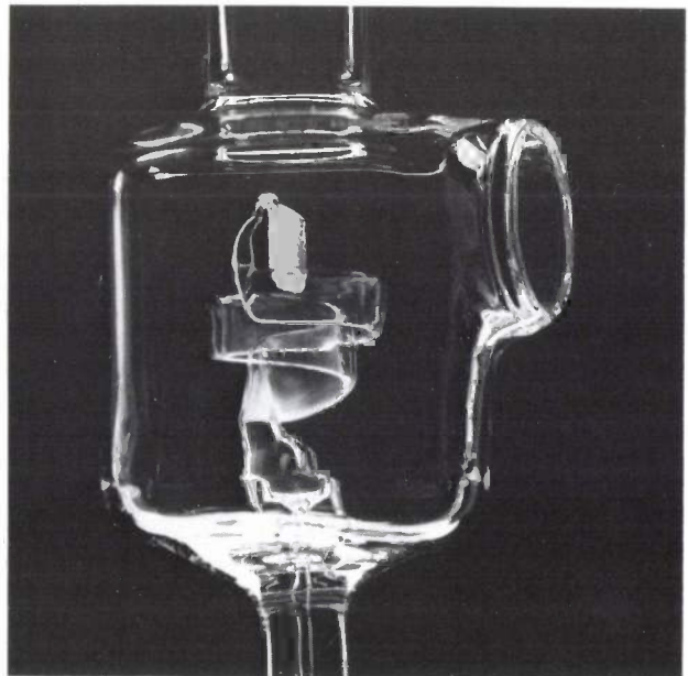
Fig. 2. The Bourdon gauge used in the instrument. The gauge consists of a spiral with a single turn, made of flat silica-glass tube with a wall thickness of 40 \mu\text{m} . At the end of this spiral is a reflecting silica-glass plate with a matt finish on the reverse side. Because of the lightweight construction the resonant frequency is higher than 500 Hz. On the left-hand side of the gauge there is a window for the incident and reflected laser beams.
