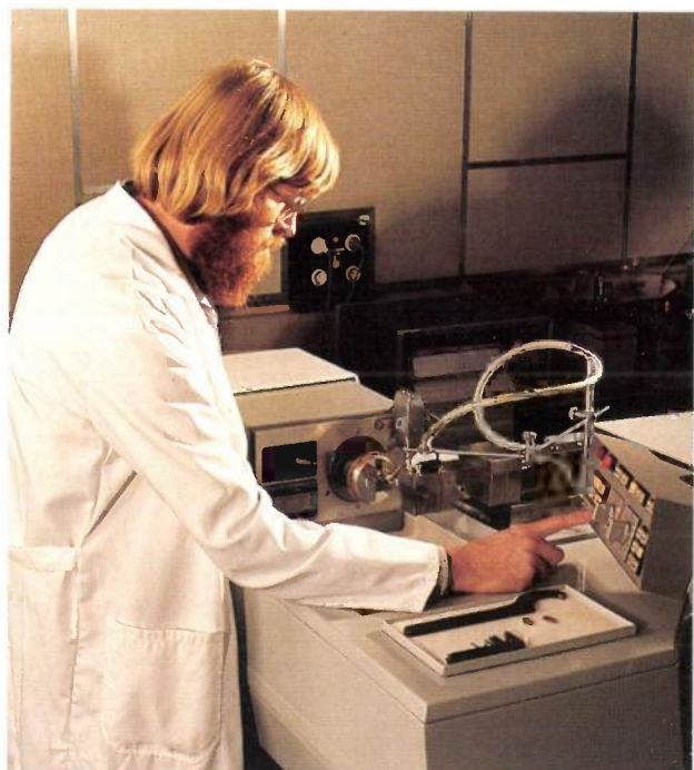
Fig. 6. The photograph shows a technician working with COLATH. The small manual control panel on the machine (right) is useful for work that has to be kept under direct observation.
