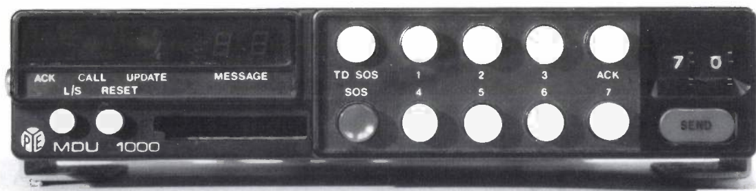
Fig. 1. Pye MDU 1000 mobile data unit, for operation with the DS 1000 vehicle-availability system. A hundred pre-numbered messages can be sent ( SEND ) and received ( MESSAGE ). The status of the vehicle can be reported by using ten other pushbuttons — 'busy', 'free', 'on watch', etc.; these messages are sent automatically in response to a call from the base station. An identity-code card is inserted in the slot at lower left.
