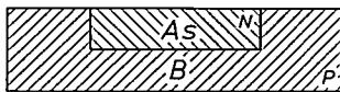
Fig. 23. Diagram of a P-N junction that can be produced in silicon by implantation of boron and arsenic.
