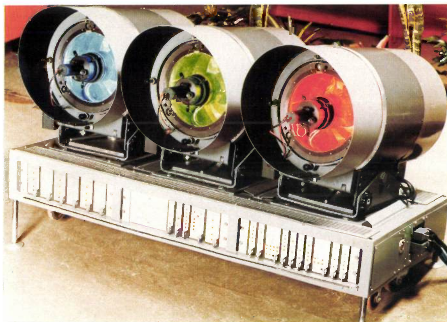
Fig. 1. The Philips professional mammoth TV projector. This is fitted with projection tubes with a diameter of 125 mm, a mirror with a diameter of 400 mm and a correction plate of 280 mm. The diagonal of the projected picture can be given any value between 1.8 and 7.5 m.
