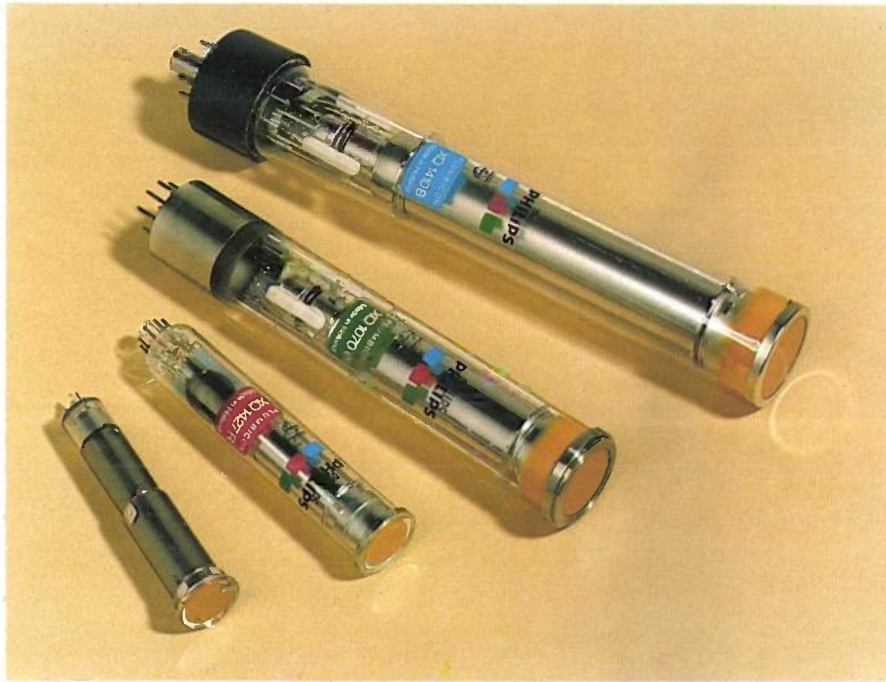
Fig. 15. Photograph of the experimental camera tube in fig. 14 and three other types.
