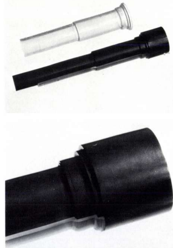
Fig. 12. Above: Photograph of a glass envelope, vacuum-formed on a profiled metal mandrel, and the mandrel, inside a half-section of the envelope. Below: A detail to illustrate the very close fit.
