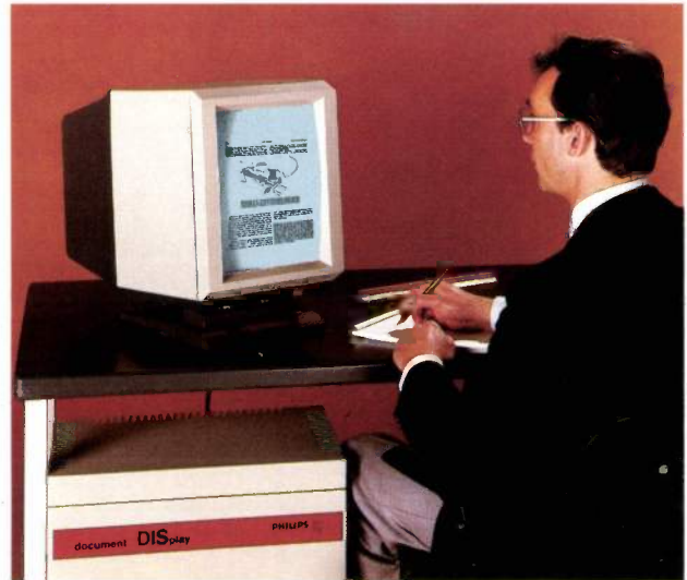
Fig. 13. The document-display screen with refresh memory. The angle of the document-display screen on the desk can be varied; the electronic circuits for the refresh memory are located below the desk.
