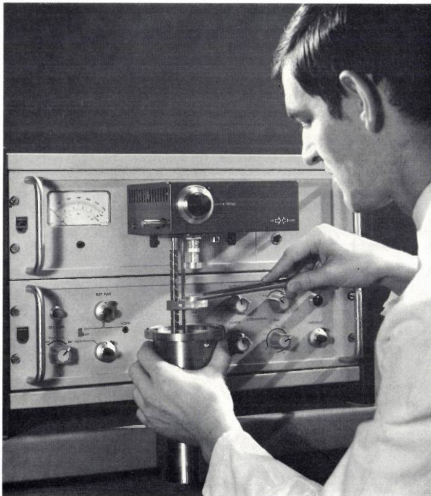
Fig. 10. An \alpha -particle spectrometer in use. The vacuum cylinder has been removed and a radiation source is being placed on the specimen holder. The height of the specimen holder can be adjusted under vacuum by means of the calibrated knob in front of the instrument. The detector is seen above the specimen holder. The meter on the left of the instrument can be used to indicate the pressure in the vacuum chamber.
