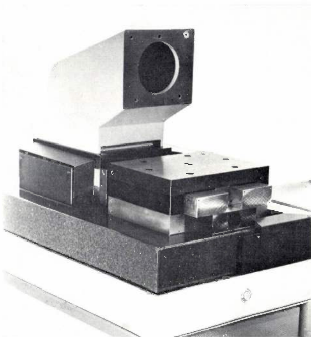
Fig. 9. The slide systems of a six-barrel step-and-repeat camera. The carriage on which the photographic plates are mounted can be seen at the front, and the carriage at the back carries the projection systems on an arm, here already fitted.
