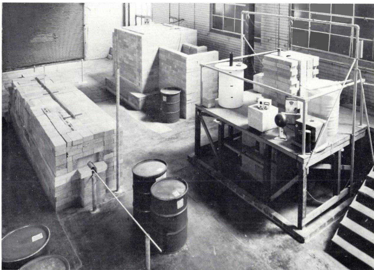
Fig. 4. Experimental rigs in the Port Melbourne laboratory for simulating bore holes. On the left is a horizontal rig 6 metres in length with removable sections to simulate mineralized zones 50 cm wide and spaced 1 m apart. On the right is a rig which enables the introduction of a radioactive nuclide neutron source into a pile of suitable brickwork or into a barrel containing finely ground material.
