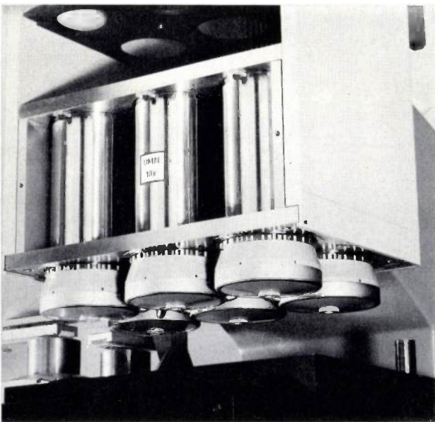
Fig. 15. Arrangement for focusing by means of air bearing. The objective tubes are mounted in diaphragm springs. The circular air bearing can be seen at the lower end of each tube.
