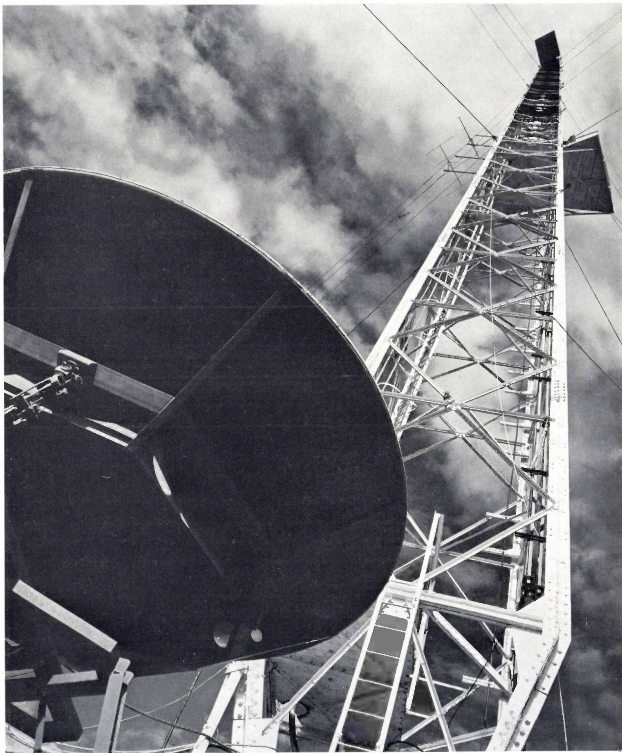
Fig. 3. Between 1950 and 1957 a considerable amount of work on "line-of-sight" microwave beam links was done at LEP in cooperation with TRT. The link between Bordeaux and the Pic du Midi (in the Pyrenées), established in 1957 using a multi-reflex klystron, at the time represented a world record: a high-definition television broadcast was transmitted directly over a distance of 213 km. The photograph shows the aerial system of the Bordeaux transmitter, with a parabolic antenna at ground level and a rectangular passive reflector at the top of the mast.
