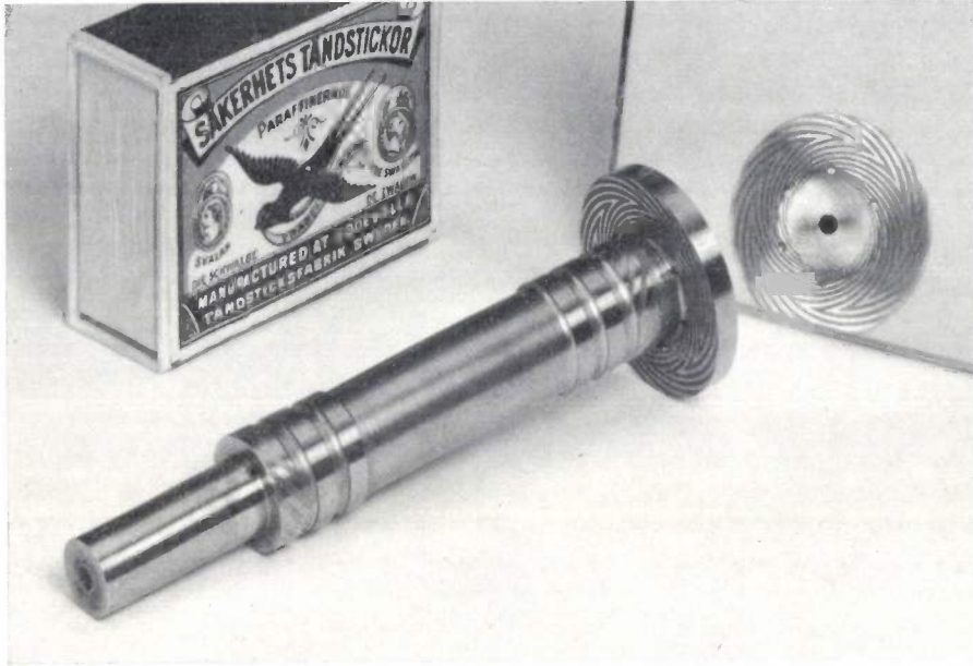
Fig. 6. The fixed shaft with thrust bearing (flange which has a spiral-groove pattern on both sides) and two journal bearings, each consisting of two sections. Helical grooves on the left and right keep the lubricant in the bearings at the correct pressure.
