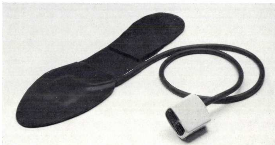
Fig. 2. Insole with flexible tube and pneumatic switch.
