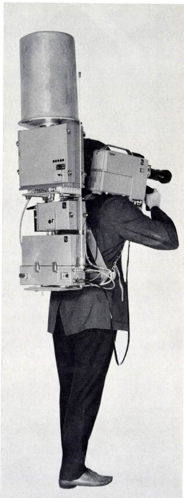
Fig. 1. Portable equipment for mobile unit. The camera, which is held on the operator's shoulder, weighs 7 kg. The equipment in the harness comprises the UHF transmitter, the intersynchronization unit and the aerial control unit with the encased directional aerial on top of it.
