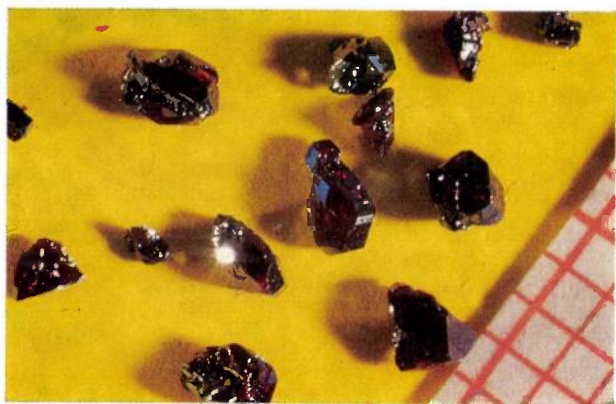
Fig. 8. Crystals of \text{CuISe}_3 obtained from \text{CuI} and \text{Se} in 5-molar \text{HI} , after cooling from 390^\circ\text{C} to 200^\circ\text{C} .
