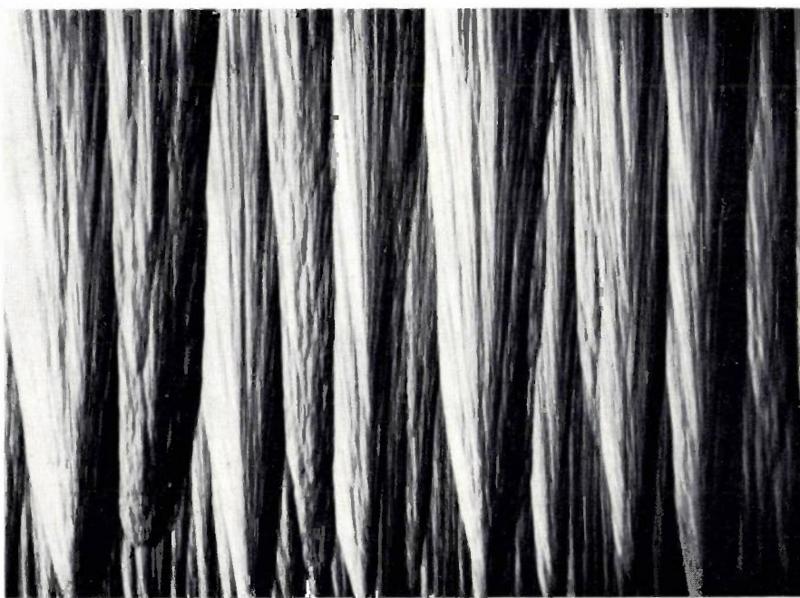
Fig. 4. Photomicrograph of a polished section through a pyrolytic graphite layer parallel to the direction of growth. The substrate is parallel to the lower edge of the photograph. Magnification 80\times .
