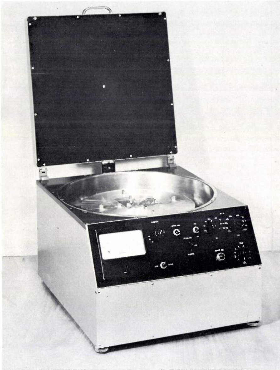
Fig. 12. Centrifugal spreader which operates either at constant speed, or at constant acceleration over a selected range. The turntable has lugs to hold the square glass plates (in three sizes). All controls are to be found on the sloping front panel. The control knob in the bottom right-hand corner ( Temp ) controls the heating element in the cover, used for drying the spread-out layer of emulsion.
