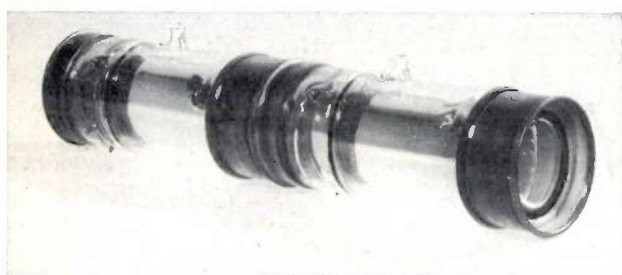
Fig. 5. An early two-stage image intensifier tube with magnetic focussing.
