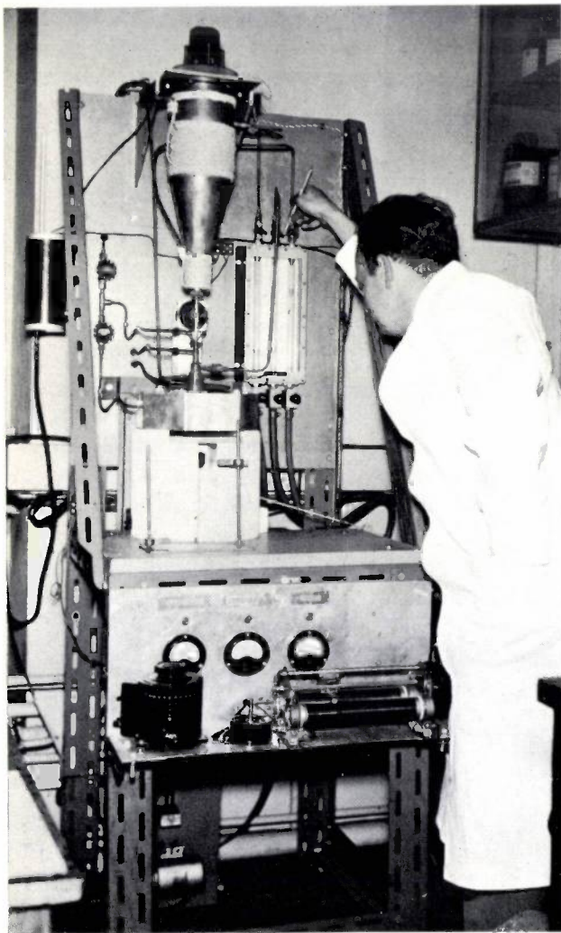
Fig. 1. The flame fusion apparatus used in the production of single crystals of manganese ferrite and associated compositions. The conical hopper contains a vibrating canister which supplies controllable amounts of powder to the vertical burner. The nozzle of the burner is directed into the top of the firebrick furnace, within which the crystal grows.
