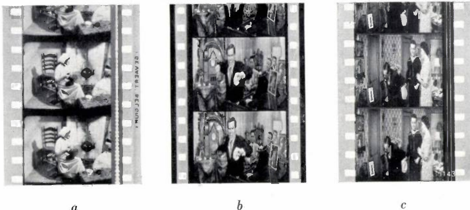
Fig. 3. Strips of 35 mm film (a) normal and (b and c) "CinemaScope". The normal 35 mm film has one optical sound-track; the 35 mm "CinemaScope" film has either four magnetic sound-tracks, two on either side of the film (b), or one optical sound-track (c). Only in the second case (b) is stereophonic reproduction possible.
