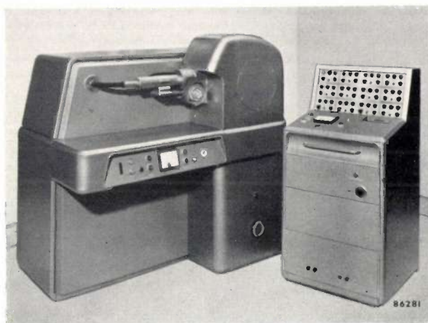
Fig. 18. The "Norelco" "Autrometer", developed for automatic X-ray spectrochemical analysis in industrial plant control. The X-ray unit is on the left and the electronic circuits unit on the right.
