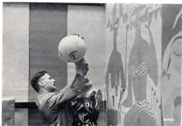
Fig. 4. Mounting the head of "Philirose". As the hair is still missing, the connecting terminals for the current supply wires can be seen on the head.
