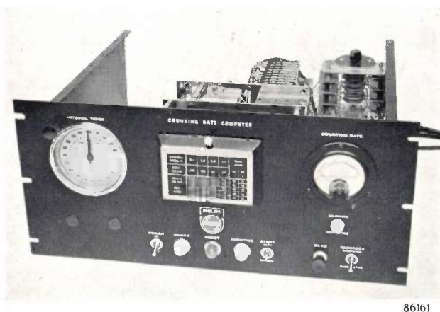
Fig. 1. Chassis and front panel of the "Norelco" counting-rate computer. This unit is placed in the electronic circuits rack of the diffractometer. The computer output can either be fed to the recorder or be read on the meter at the upper right. At the upper left a register is mounted which is not used for the computer but only in manual fixed count measurements (cf. II).
