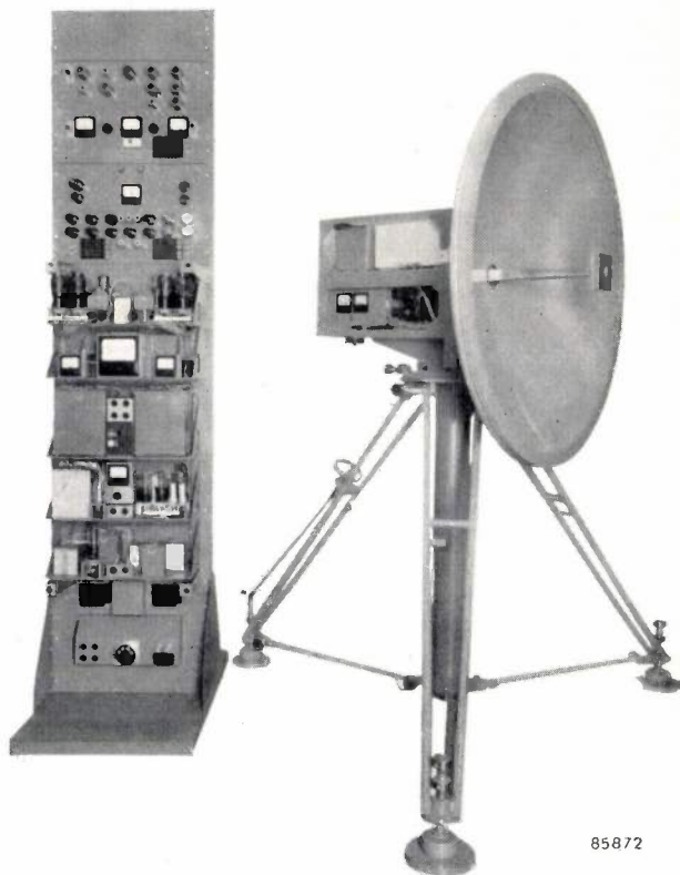
Fig. 7. The experimental transmitter for double frequency modulation. To the left is the rack, to the right, mounted on a tripod stand, the reflector assembly, containing the output stages of the transmitter.
