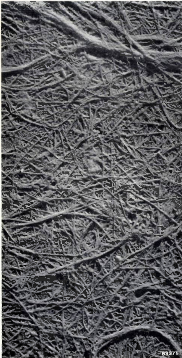
Fig. 14. Animal cellulose (Tunicine). Magnification 20 000 \times . Micrograph made with the EM 75 kV. (L. H. Bretschneider, Utrecht.)
