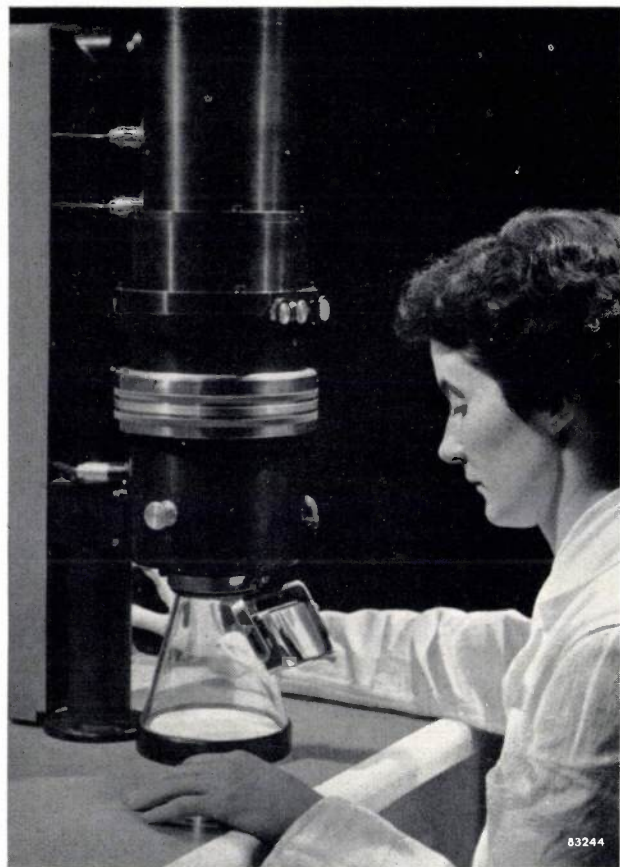
Fig. 13. The microscope tube of the EM 75 kV. By turning the milled ring which encloses the tube, the upper pole piece of the projector lens is displaced. The ring can make \frac{7}{8} of a complete turn; this causes the pole piece to move 15 mm in a vertical direction, which alters the magnification by a factor 9. The wall of the vacuum tube is here formed by a thin brass tube ( b in fig. 12), which makes a sliding fit in the other of the pole pieces, which are thus outside the vacuum.
