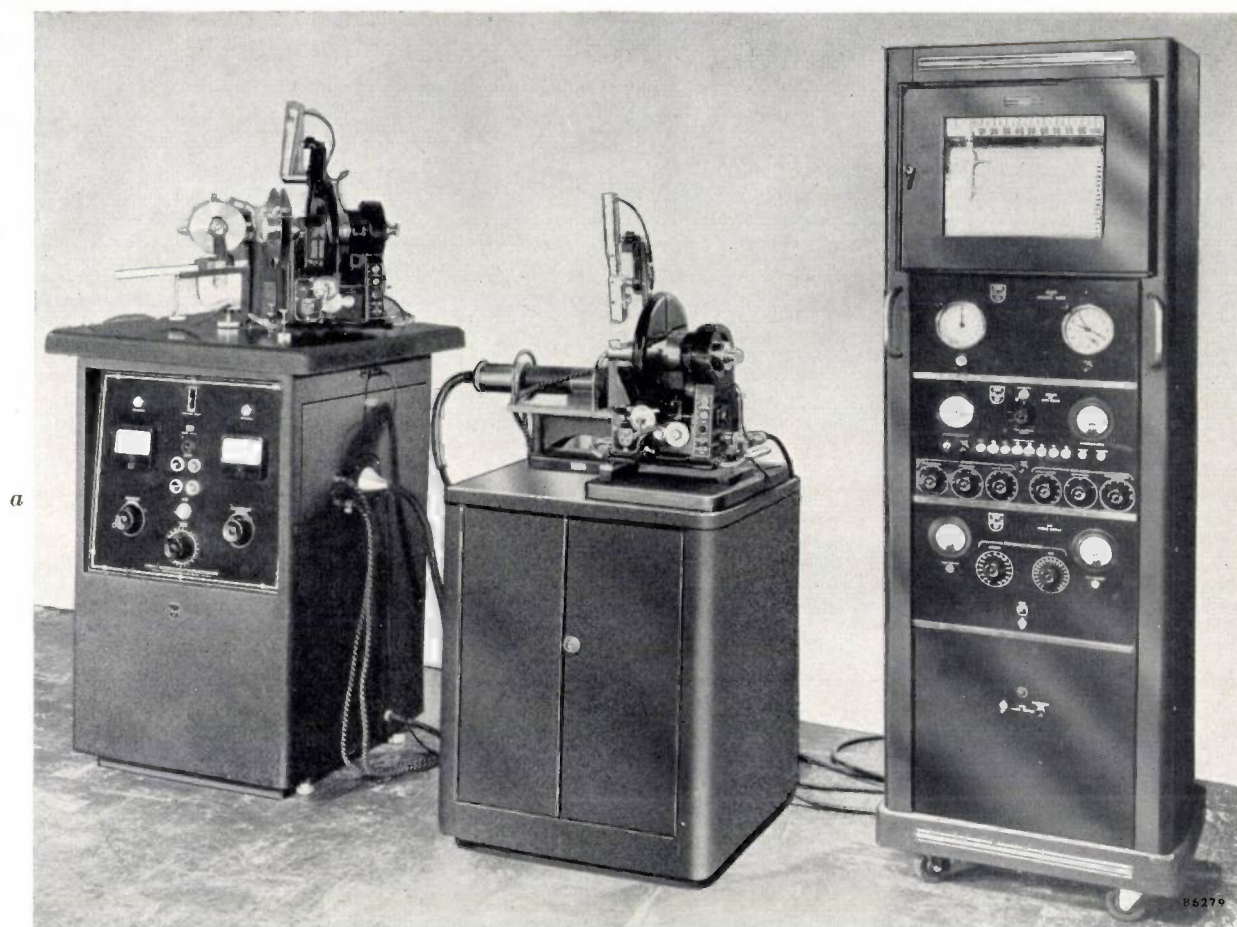
Fig. 5. a) "Norelco" equipment both for X-ray diffraction and X-ray spectrochemical analysis. The X-ray generator, with powder cameras and a goniometer for diffractometry on top of it, is shown in the left; the X-ray spectrograph for spectrochemical analysis is in the middle; the electronic circuits rack including the counting-rate meter and recorder is on the right. The same X-ray generator and electronic circuits are used for both methods but the methods cannot be used simultaneously. b) Goniometer arranged for spectrochemical analysis: X horizontally mounted X-ray tube, S specimen chamber, C analyzing crystal, P parallel slit system, D radiation detector (scintillation counter).
