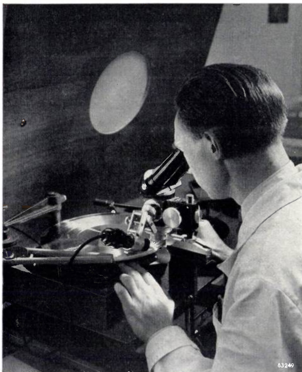
Fig. 8. Checking the positive for damage and dust particles.
