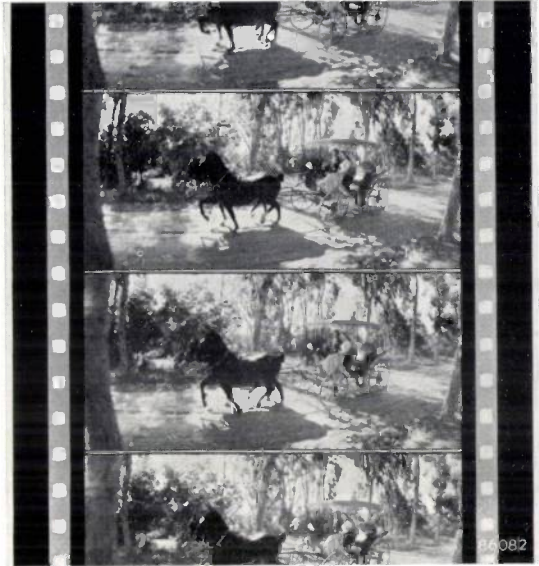
Fig. 2. Strip of 70 mm film. It has six magnetic sound-tracks, three on either side of the film. The wide black bands on the outside of the perforations carry two sound-tracks each; the narrower bands inside the perforations carry only one each. The height of the frame is equal to 5 perforations.
