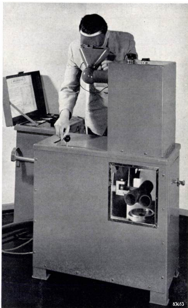
Fig. 1. Industrial radiology equipment using the image intensifier, for experiments and demonstrations. Note the beam exit aperture of the X-ray tube, radiating vertically upwards, behind the lead glass window. Above it is the work to be examined, in this case a welded Y-joint. The image intensifier, mounted in a box on top of the apparatus, is provided with an angled optical system. The two handles seen on the left of the apparatus, are manipulated by the observer to locate the work as required.
