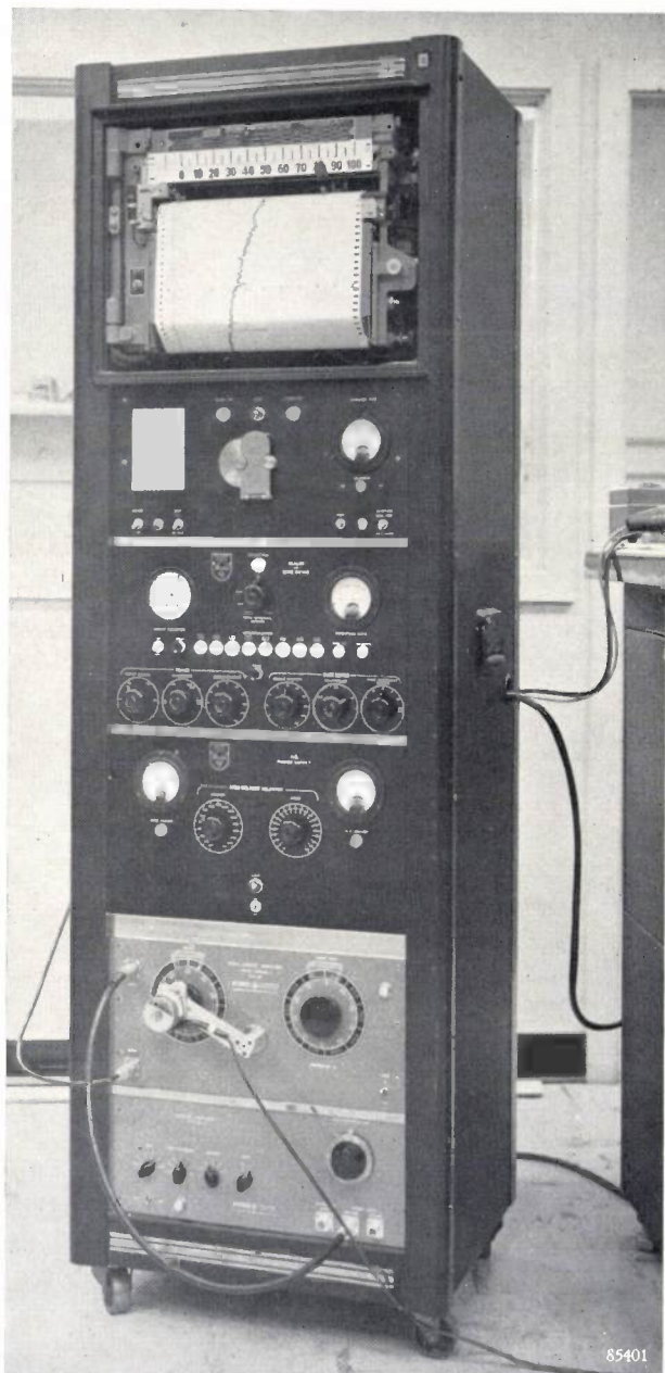
Fig. 1. Rack containing circuitry and accessories for the measuring and recording of diffracted X-ray intensities with the "Norelco" X-ray diffractometer.
