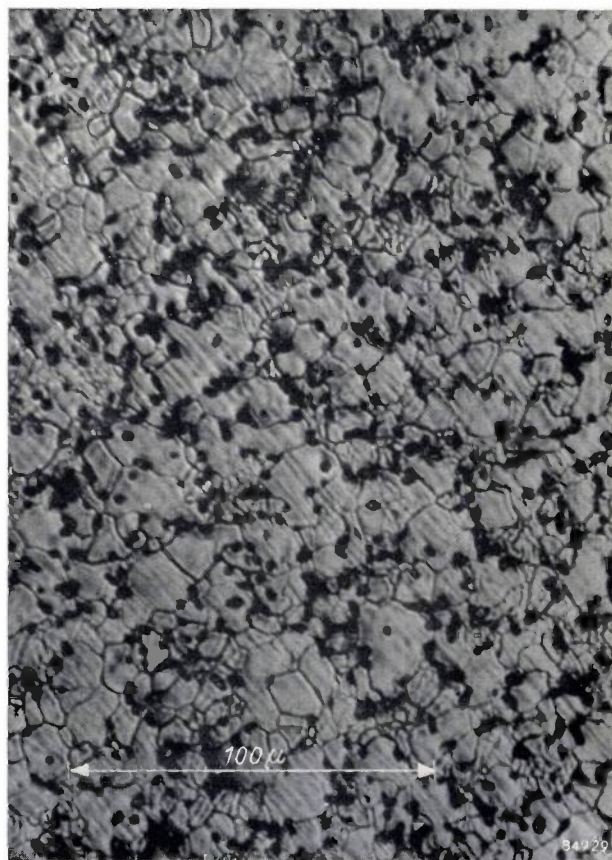
Fig. 2. Photomicrograph showing a polished section of the tungsten surface after the volatilization of the copper. The average pore size is of the order of a few microns, the pore separation varying between a few microns and a few tens of microns. (Such small pore distances are desirable for the surface of dispenser cathodes 7 .)
