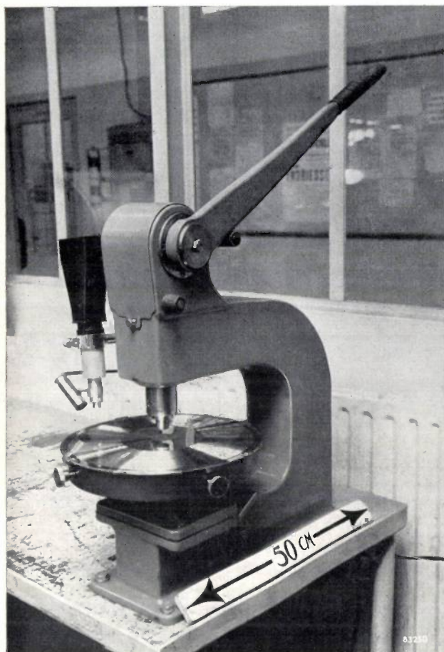
Fig. 10. Centring a matrix. The latter is loosely champed to a rotatable table. The position is altered until on turning the table, the grooves, viewed through a microscope, are seen to move in one direction only (either inwards or outwards). The lever is then pulled down, punching out the centre hole.
