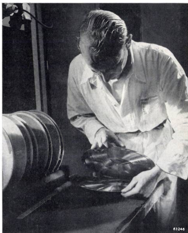
Fig. 9. Separation of the positive and the electroformed stamper.
