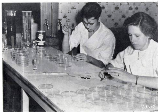
Fig. 1. Irrigation of petri dishes with a solution of the compound to be investigated for tests on flies and grain-weevils. The solvent (usually acetone) is allowed to evaporate, leaving behind a known quantity of the compound in a thin layer.
