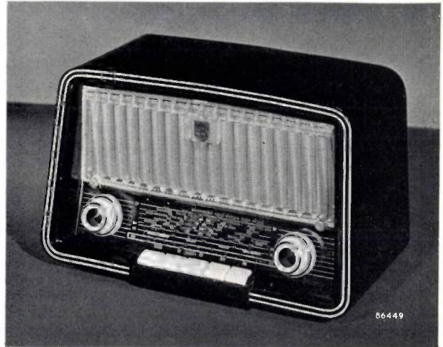
Fig. 5. Receiver with separate tuning knobs for AM and FM (type BX 253 U). In the right is a double knob for tuning; the front knob is used for AM and the rear for FM. The left-hand knob is also double; the front knob is used for the volume and the rear one for the tone control. The buttons in the centre are (from left to right); on/off switch, long wave, short wave, medium wave, and F.M. reception. For gramophone reproduction, the long and the short wave buttons are pressed in together.
