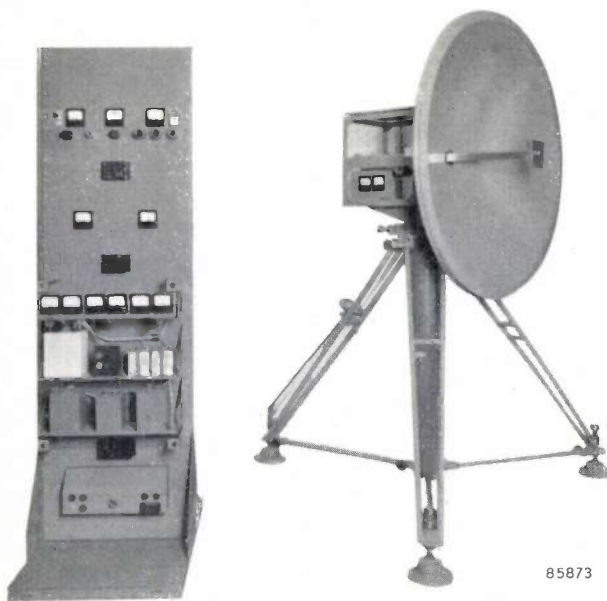
Fig. 9. The experimental receiver for double frequency modulation. To the left is the rack, to the right, mounted on a tripod stand, the reflector assembly containing the first stage of the receiver.
