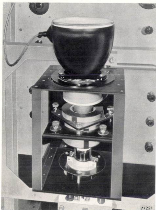
Fig. 2. The cathode-ray tube for the flying-spot scanner (type No. MC 13-16), fitted with its focusing and deflecting coils.
