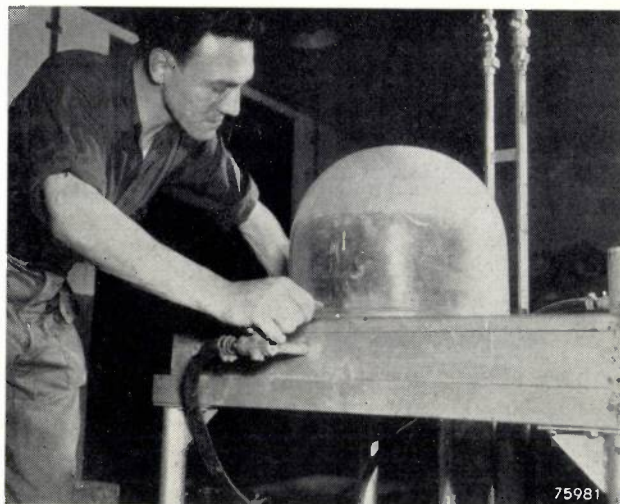
Fig. 13. Before vibration the air bubbles are removed from the moulding mass by placing a vacuum bell over the box and connecting it for a time with a vacuum pump.
