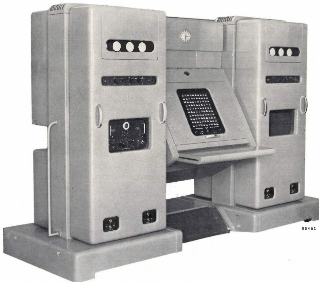
Fig. 14. The main assembly. Front view showing in the centre the register and control desk. At the top of the left and right sections are the delay unit monitor tubes; below them are the delay unit control panels. Half way down on the left section is a total count scaler (on the right there is a position for another scaler). At the bottom, left and right, are the power supply control panels.
