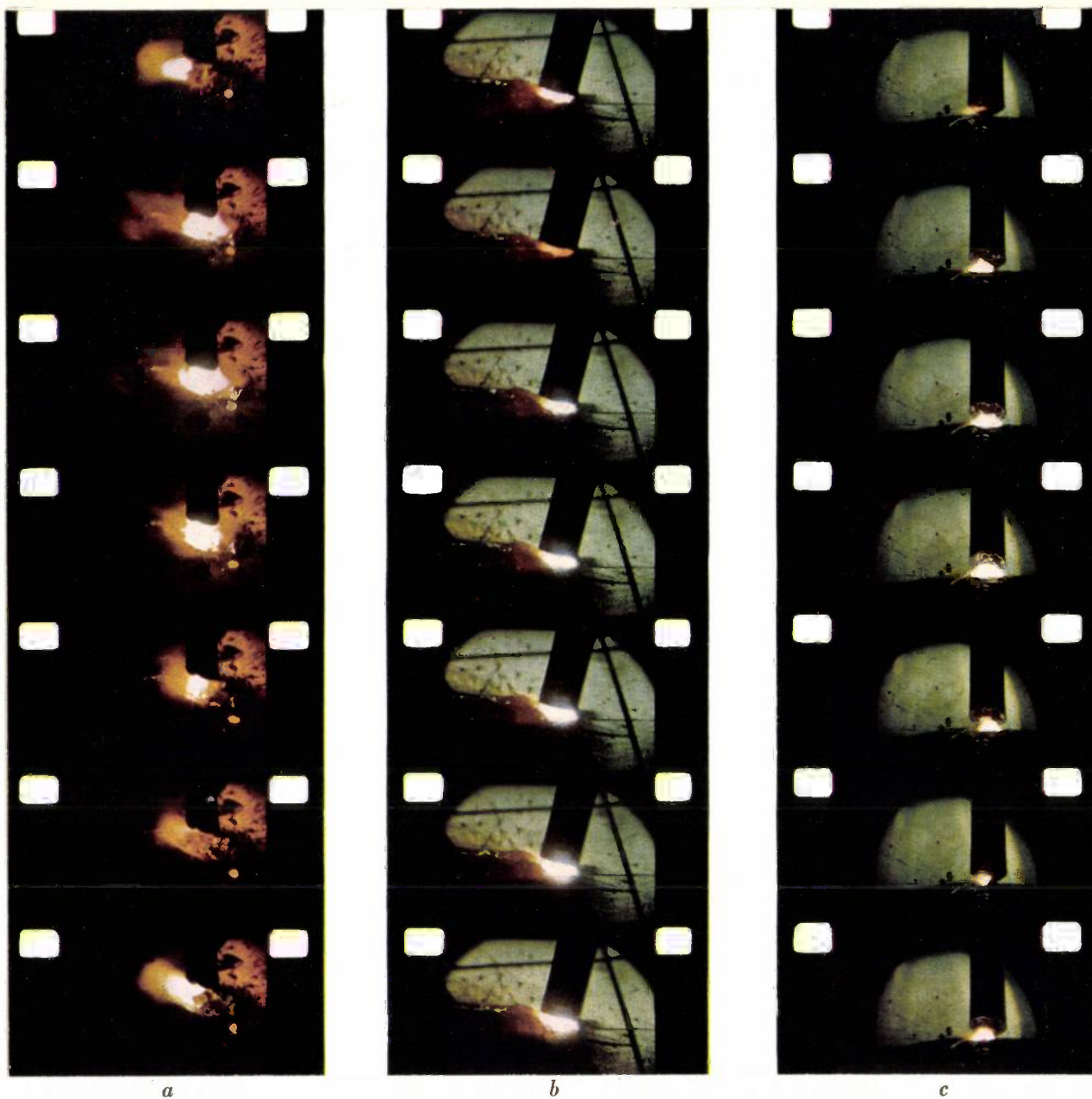
Fig. 7. Extracts (not sequential) from three colour films of arc welding with A.C. The differences in colour between the films are due to the use of different filters. (a) and (b) were filmed with the set-up shown in fig. 8; (c) with that of fig. 9.
