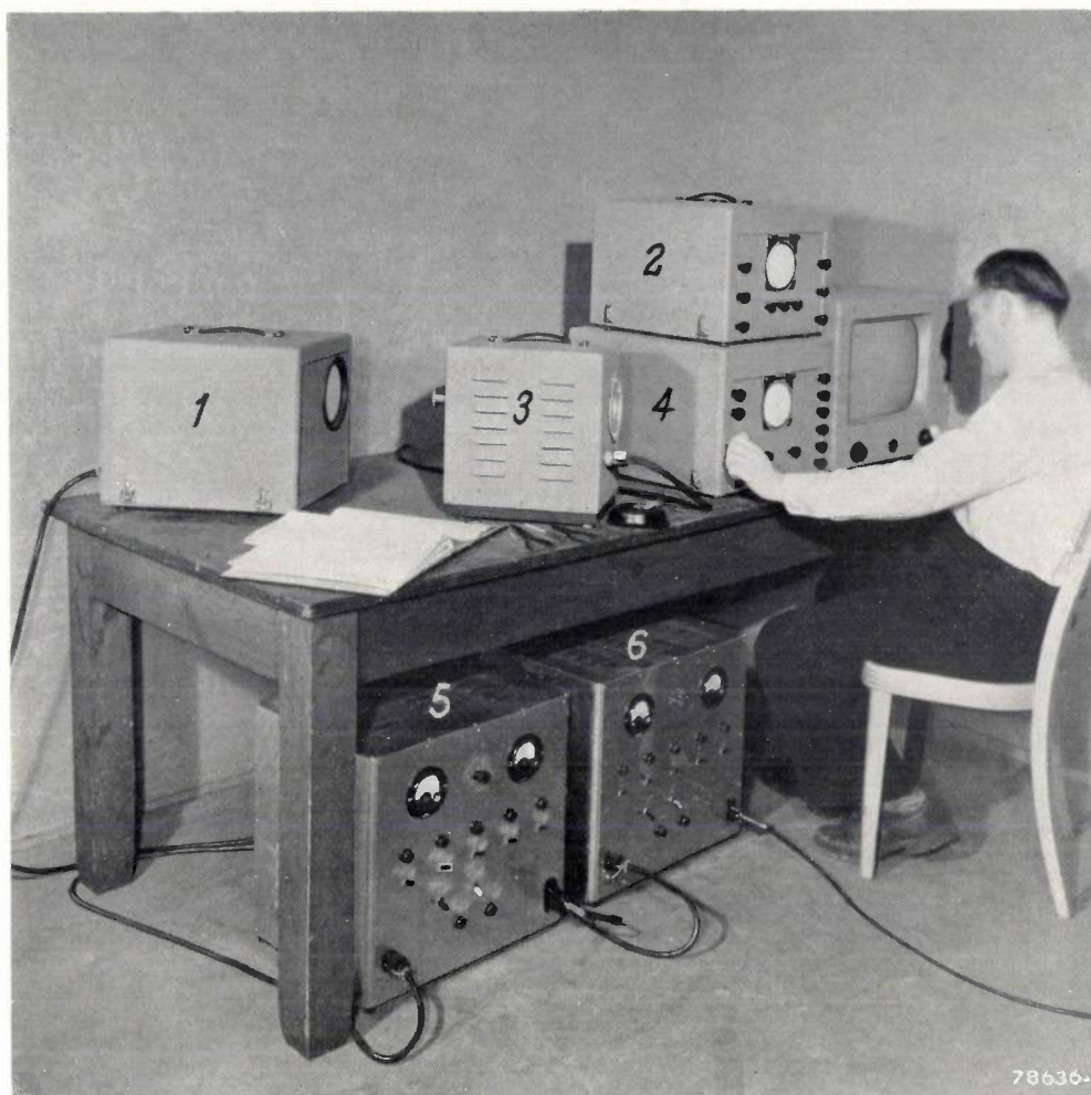
Fig. 7. The six portable units, constituting the line converter used at Breda. Unit 1 contains the picture tube, the video-output amplifier and the oscillator for spot-wobbling. Unit 2 contains the first video amplifier, the saw-tooth generators for the picture tube and the controls. Unit 3 contains the camera and its image iconoscope, type 5854, two output valves for the deflection currents and a pre-amplifier for the picture signal. Unit 4 houses the second picture-signal amplifier, the saw-tooth generators and the controls. 5 and 6 are power-supply units. To the extreme right is a monitor.
