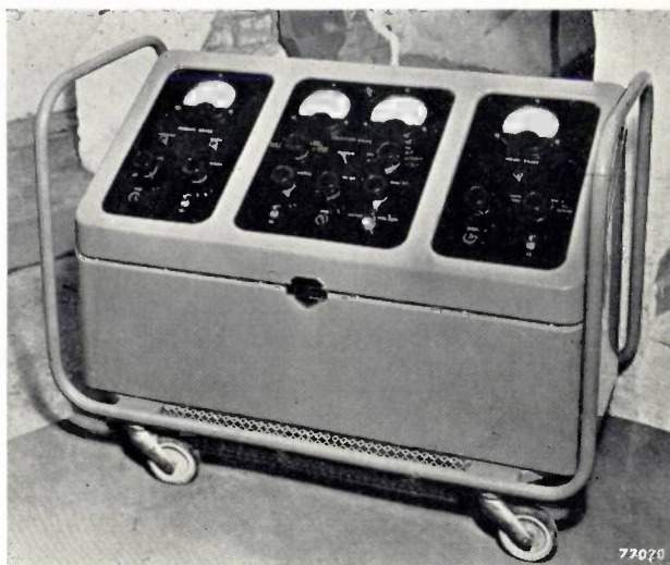
Fig. 16. Trolley housing the control units for all vacuum gauges (Pirani, Philips and triode ionization gauge).
