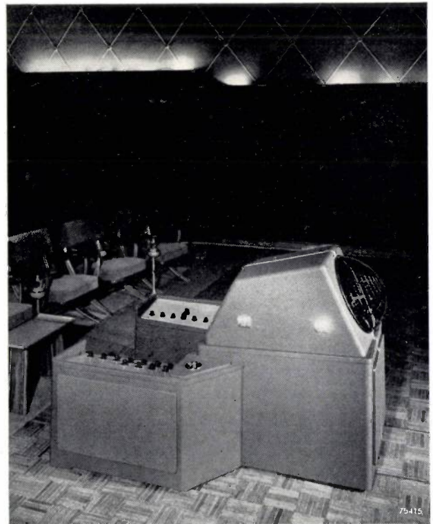
Fig. 5. The Mammoth projector (Type EL 5750) mounted in front of the first row of seats in a hall. The projectionist takes his place behind the main body, between the "wings". The unit is so low that projectionist and public have an unobstructed view of the screen.
