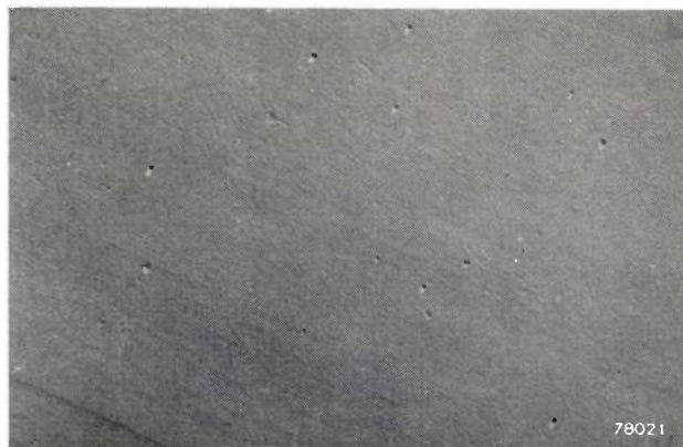
Fig. 1. Elementary lines on the surface of an aluminium crystal which has been stretched by a few per cent. Magnification 20,000x (Figs. 1 and 2 are taken from H. Wilsdorf and D. Kuhlmann-Wilsdorf, Z. angew. Physik 4, 341, 1952.)
