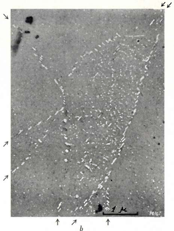
Fig. 5a) Geometrical representation of dislocations at the boundaries between two crystals. (Vide J. M. Burgers, Kon. Ned. Akad. Amst. 42 , 293, 1939.) b) "Developed" dislocations of the kind depicted in a). The distances are as anticipated from the observed disorientation angle of the adjacent crystals. The arrows indicate the crystal boundaries. (R. Castaing and A. Guinier, Comptes rendus 228 , 2033-2035, 1945.)
