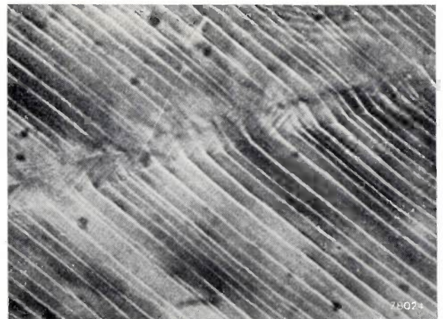
Fig. 6. Polygonized deformation band on the surface of an aluminium crystal elongated 31% and annealed for 1 hour at 450 °C after stretching. Magnification approx. 200x.
