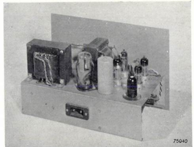
Fig. 6. View of the oscillator section of the metal-detector for bulk materials.
