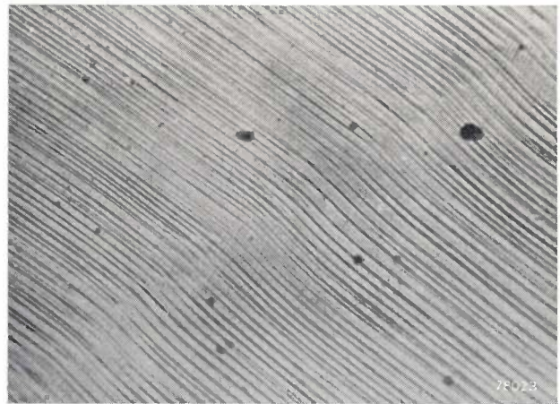
Fig. 4. Deformation band on the surface of an aluminium crystal with 20% extension. (Magnification 250 \times ). Note the curvature of the slip lines. (Figs. 4, 6 and 8 are taken from R. W. Cahn, J. Inst. Metals 79, 129, 1951.)
