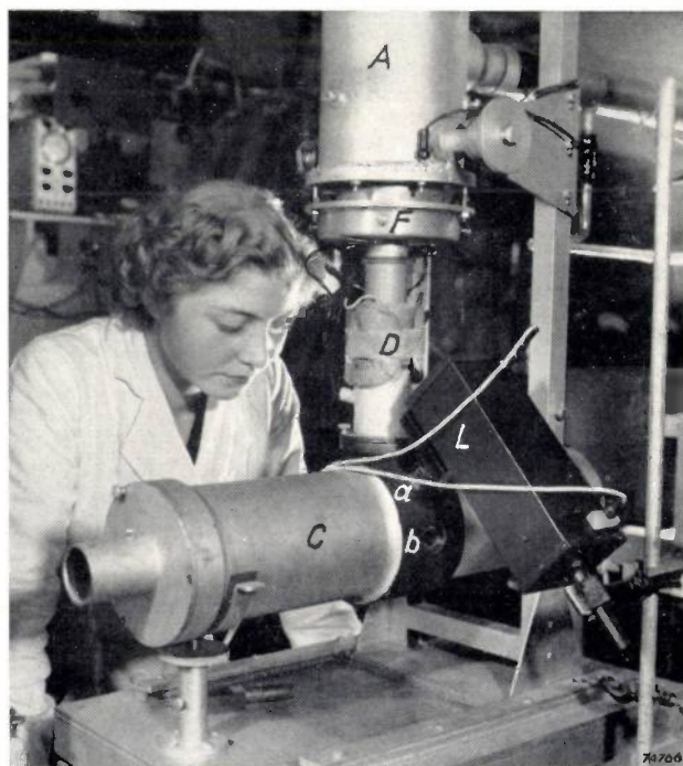
Fig. 1 a ) Diagram of apparatus for the measurement of fluorescent efficiency. A metal chamber, h anode, f filament, g cap, p pump connection, F focusing coil, D deflection coils, B glass tube, C metal cylinder, P target plate, a , b , c and d quartz windows. M microammeter. b ) Photograph of the equipment. L box containing photoelectric cell.
