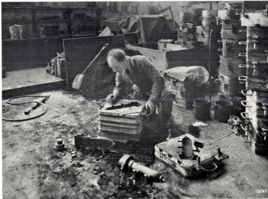
Fig. 1. Upper and lower boxes of a sand mould. The wooden pattern can be seen in the foreground. In the upper box the "gate" or "sprue" can be seen through which the metal is poured. (This photo, taken in the Reineveld Engineering Works at Delft, was supplied by the Casting Research Centre, National Council for Industrial Research, Netherlands.)
