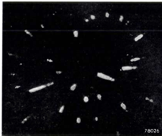
Fig. 8. a) Transmission Laue photograph of aluminium crystal elongated by 7%. The deformation is revealed by the elongated diffraction streaks (asterisms). b) The same crystal after 36 hours annealing at 590 °C. The asterisms are now broken up into discrete spots.
