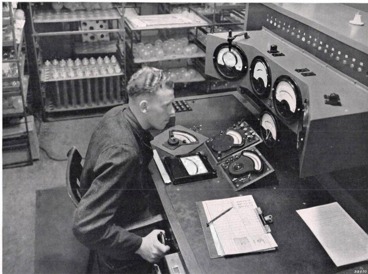
Fig. 4. Measuring table of the installation. The vertically placed instruments measure the mains voltage and the current (when a transformer is used, primary and secondary separately). The instruments placed obliquely on the table measure the total power. The left-hand horizontal meter measures the photo-current, the right-hand one the voltage on the contacts of the lamp. To the right on the table may be seen the handles of the rotating switches, each of which serves part of the photometer cabinets. To the left on the table a series of switches for the photo-elements of the different photometer chambers. Above the meters are the neon lamps which glow when the heating time of the corresponding lamp has ended.
