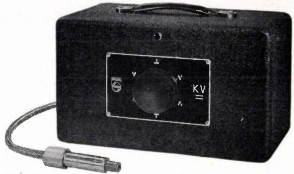
Fig. 8. The 5 000-volt supply apparatus GM 4 198 for the post-acceleration tubes of the cathode ray oscillograph GM 3 156. The apparatus contains a high-voltage transformer, a rectifier valve and a filter for smoothing the D.C. voltage obtained. As may be seen it can be set at five different voltages with the help of a switch.
