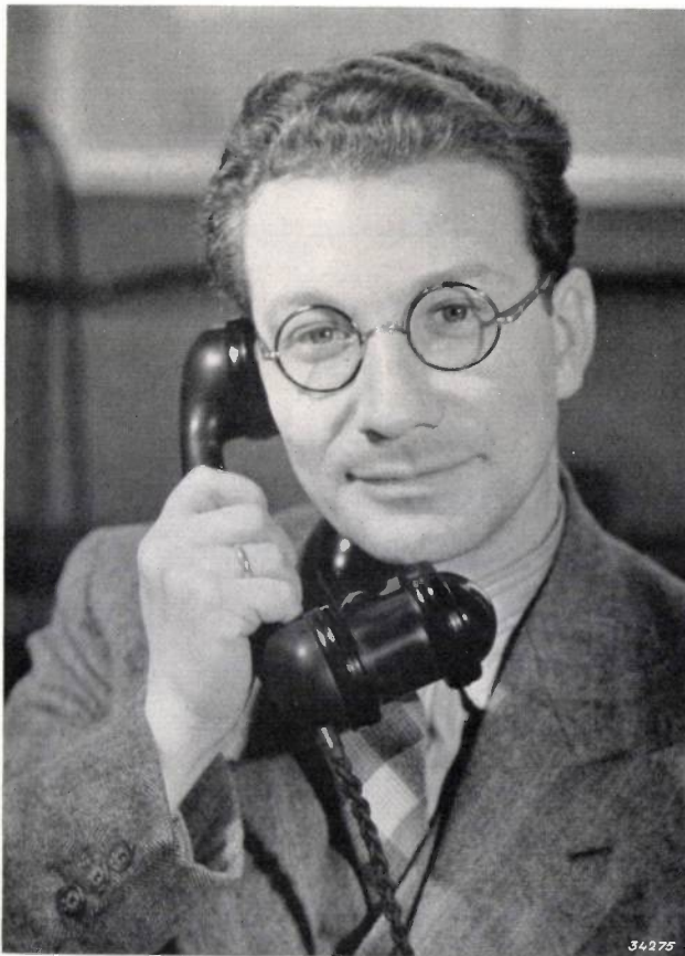
Fig. 13. When the arms to which the laryngophone is attached are turned into such a position that the laryngophone rests against the throat when the apparatus is held in the ordinary way, the air microphone is automatically disconnected by a switch situated in the intermediate section.
