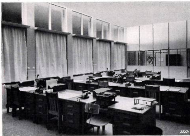
Fig. 3. Illumination of a long narrow office room by means of coves along a side wall. The absence of lighting fixtures hanging from the ceiling makes possible a clear view of the whole room.
