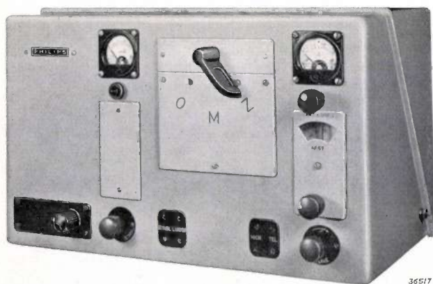
Fig. 8. The transmitter-receiver DR 38. In the middle, the switch with three positions for reception, measuring and transmitting. Below, the connections for the tele-microphone and the call loud speaker.
