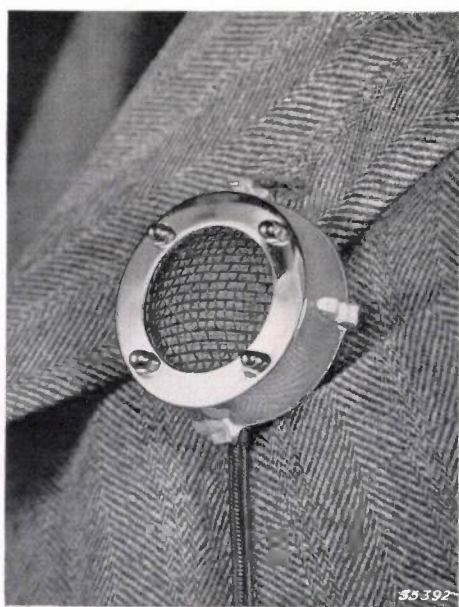
Fig. 13. Carbon microphone, type 4225, special model for reporters. The microphone can be hung in the buttonhole of the coat.
