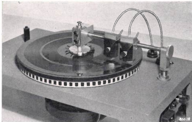
Fig. 2. Apparatus for sound recording on discs, designed for stereophonic recording. Two sound track cutters are mounted on the transport shaft, each of which is fed from one of the two microphones and which cut a sound track in the inner and outer zones, respectively, of the disc.
