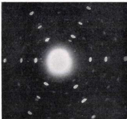
Fig. 2. Spot pattern obtained by the diffraction of a beam of X-rays through a single crystal (Laue photograph).
