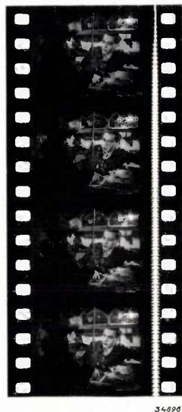
Fig. 2. Strip of film with pictures and sound track (recorded with amplitude modulation). The height of a frame corresponds to three sprocket-holes.
