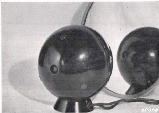
Fig. 7. A sphere with a diameter of about 22 cm may be used as an "artificial head". The microphones are situated at the extremities of a horizontal diameter.
