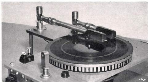
Fig. 6. Arrangement for playing stereophonic records. The arm of the outer pickup is shorter than that of the inner pickup according to a definite relation (equation (5)).
