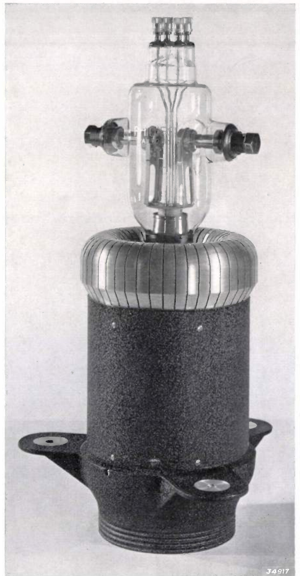
Fig. 7. The transmitting triode type TAL 12/10 (12 kV, 10 kW) with four connecting wires for the filament which is heated with two-phase alternating current.
