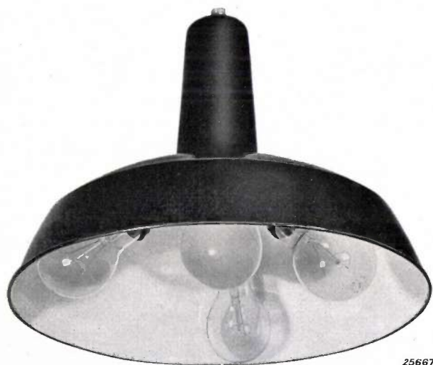
Fig. 5. Blended-light fitting. Enamelled reflector for workshop illumination, containing three ordinary electric lamps and one mercury lamp.
