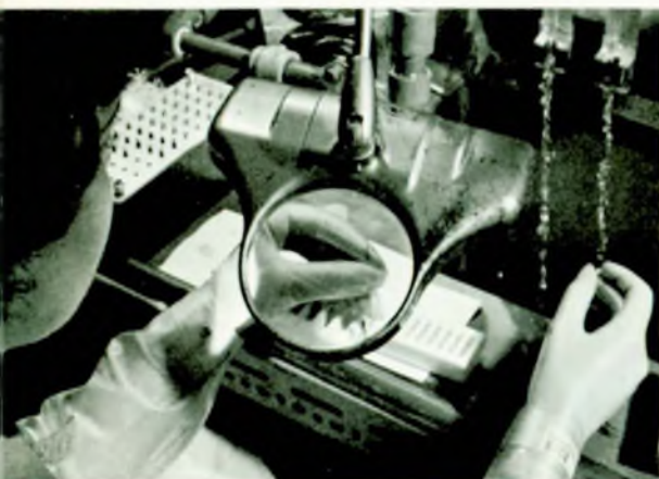
Surface Treatment—Clean-up Etch for SBT Transistor
