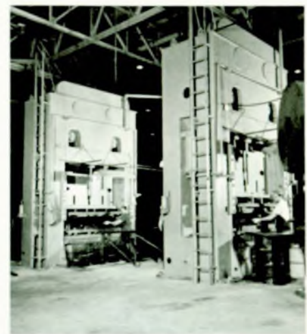
Refrigerator parts are stamped in huge presses at Connersville
