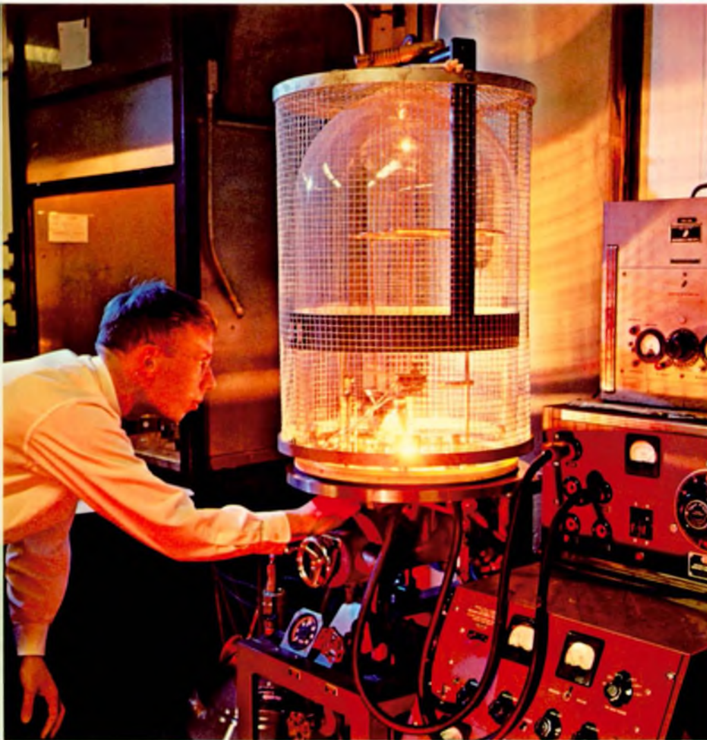
Evacuated bell jar for thin film deposition
