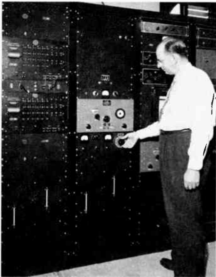
Figure 13. NBS Primary Resonator Frequency Standard. Temperature-controlled quartz crystals are made to resonate at a frequency of 100 kc. Several of the oscillators are offset from 100 kc. by a small number of cycles to permit comparison measurements by dual electronic counters. A variable oscillator is also employed in the comparison measurements. The accuracy of this system is more constant than the rotation of the earth, the present National standard of time. Therefore, deviation of the oscillator frequency (and, therefore, that transmitted by WWV) from the mean sidereal day must be computed. These variations are periodically issued as corrections to the NBS frequency standard utilized by science, industry, and commerce.
