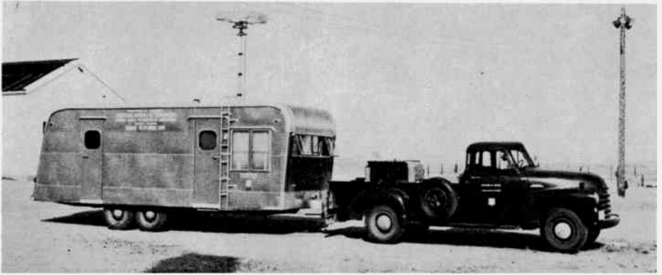
Figure 6. Mobile Research Unit Used by the National Bureau of Standards to Measure the Field Strength of Radio Signals. Mobile units such as these have been sent to Pikes Peak to determine range of transmitted signals from installations in the general area. Others have cruised in service areas common to several transmitters to determine the amount of interference offered by each station. The antenna (on top of trailer) can be raised to a height of 30 feet by remote control while the unit is in motion.
