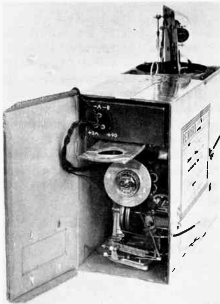
Figure 2. The Radiosonde, Originally Developed for the Navy by the National Bureau of Standards in 1936, Suspended from a Free Balloon, Telemeters Information on Upper-Air Pressure, Temperature, and Humidity. The instrument is in general use by the Navy, Army, Coast Guard, and Weather Bureau for collecting meteorological data employed in weather forecasting, and has replaced the airplane for obtaining information of this type. The radiosonde employs a modulator and oscillator, the ultra-high-frequency output of which is controlled by special resistors that are sensitive to changes in atmospheric phenomena. The changes in modulation frequency are thus measures of the phenomena studied.
