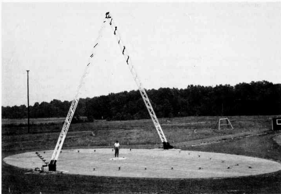
Figure 5. NBS Model Antenna Range. This range is believed to be the largest of its kind designed to measure antenna radiation patterns in the vertical plane. The inverted-V structure supports a self-contained target transmitter at the vertex and is designed to move in a 180-degree arc. The antenna to be tested is placed at the center of the oval-shaped ground plane. The model techniques that are used permit an investigation of antenna characteristics in the 1-to-25-mc. region while actually operating at frequencies between 60 and 1500 mc.
