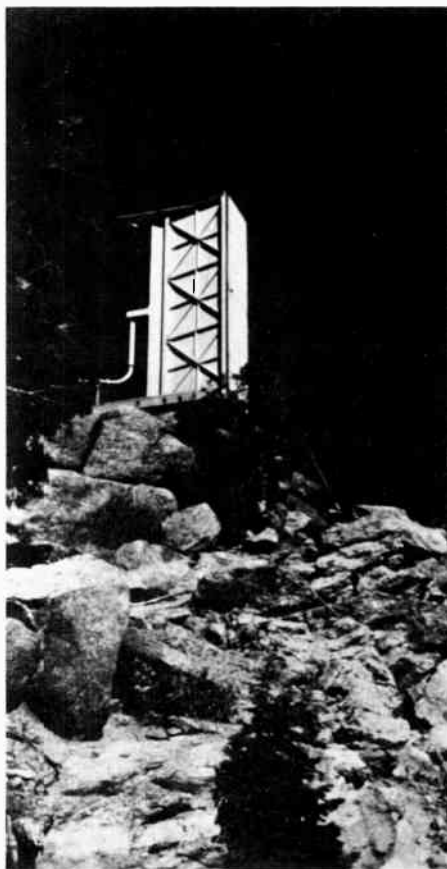
Figure 9. Semipyramidal Horn Antenna Located on Top of Cheyenne Mountain, Colorado. The radiator is used in experiments designed to determine the conditions of the troposphere causing reliable reception of signals more than 500 miles from the transmitter. This antenna radiates 1.6 megawatts of effective power at a frequency of 1046 mc.
