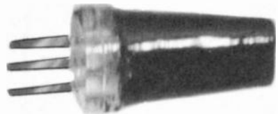
Figure 35. Completely Assembled Fused-Junction Transistor
