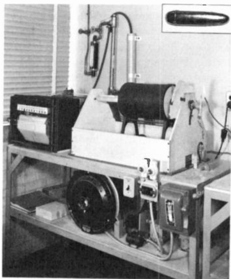
Figure 7. Germanium Reduction Furnace
