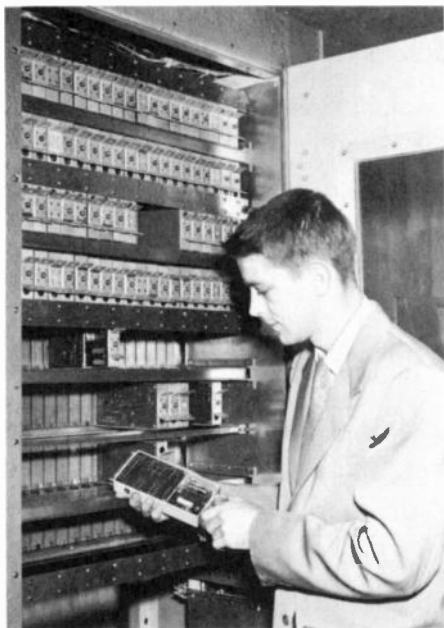
Figure 1. Plugging One of New NBS "Packages" into Electronic Computer Rack at National Bureau of Standards
