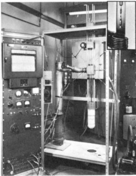
Figure 8. Crystal Pulling Furnace Setup (The equipment on the right is an induction heater used to energize the coil around the quartz tube. Monitoring equipment is contained in the rack at the left. The inset shows a pulled ingot just prior to removal from the furnace.)
