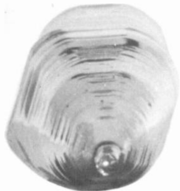
Figure 12. Seed-End View of Pulled Single Crystal
