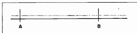
Figure 7. Random Distribution of Dots Over an Interval, Showing Method of Determining Dot Density. (The average density of dots per unit length at any point between A and B may be assumed to be: D_{AB} = N_{AB}/L_{AB} , where D_{AB} = average dot density, L_{AB} = length of interval from A to B, and N_{AB} = number of dots between A and B.)
