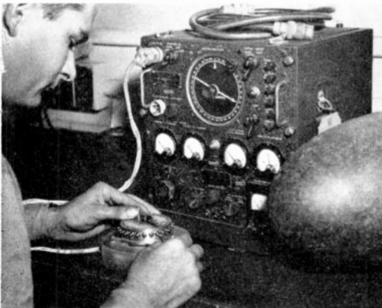
Figure 7. Adjusting a Loop Compensator, Using Jig and Test Set
