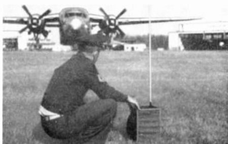
Figure 4. Target Signal Generator Being Used for Line Testing of Aircraft
