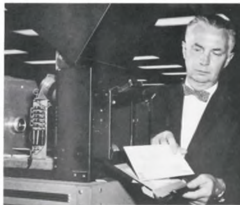
Chester P. Woodward, director of engineering for the department, is seen inserting a letter to be read by the scanner unit. The unit is capable of reading machine printed alphanumeric symbols. The flying spot beam which scans the letter is focused through the lens in the center and emanates from the cathode ray tube at the left.
