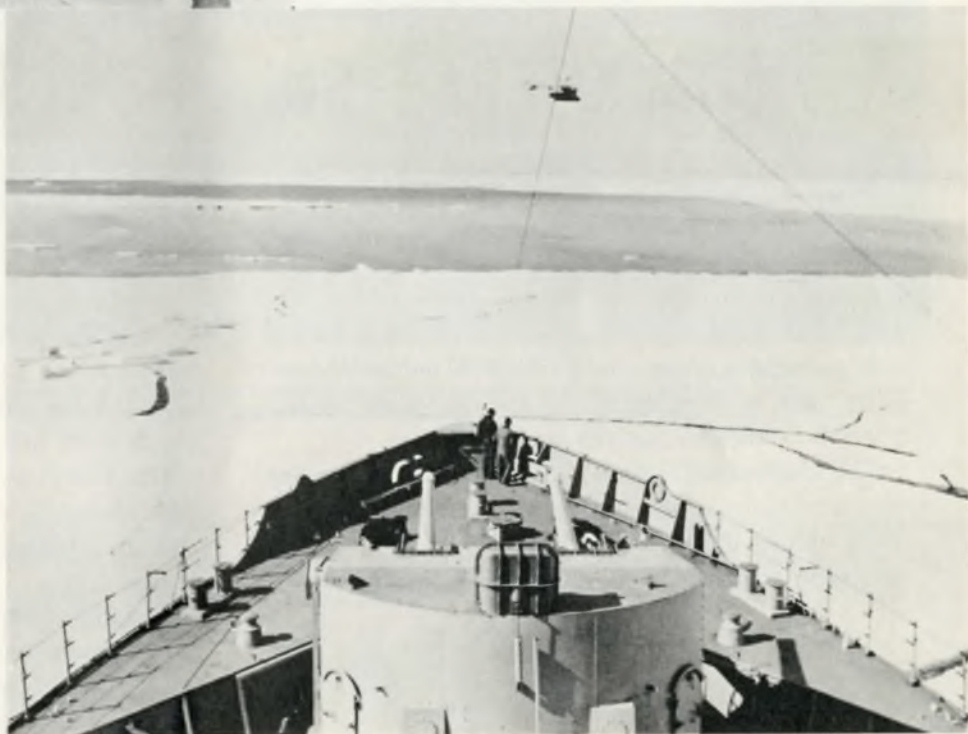
FLYING TV STATION —Bow of the Navy's most powerful icebreaker, USS Glacier, smashes through a field of ice in Melville Bay off the coast of Greenland as a Navy helicopter uses Philco airborne television for observing ice conditions ahead of the ship. This vital information is instantly relayed back to the icebreaker.
