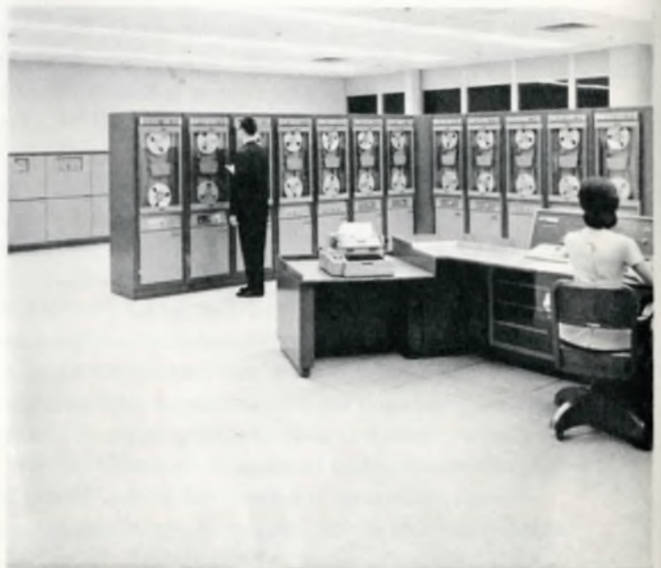
General view of the demonstration room for the Philco 2000 electronic data processing system. The central computer and console typewriter is in the right foreground; the magnetic tapes are in the center and the high speed printer and printer controller are at the right.
