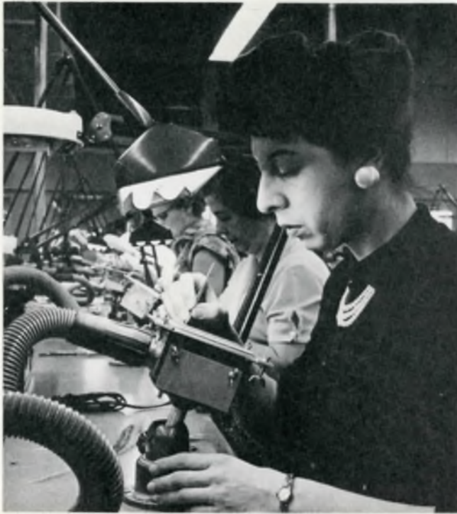
The wiring of the magnetic core plane for an electronic data processing system is shown being done here at Philco's new Computer Division facility at Willow Grove, Pa. Each core plane has 4,096 minute magnetic cores which must be assembled and wired together. The magnetic core memory in Philco 2000 computer systems is available in 10 micro-second or two micro-second access time. The production assembly line here is one of many such lines in the Computer Division's new 210,000 square foot facility.
