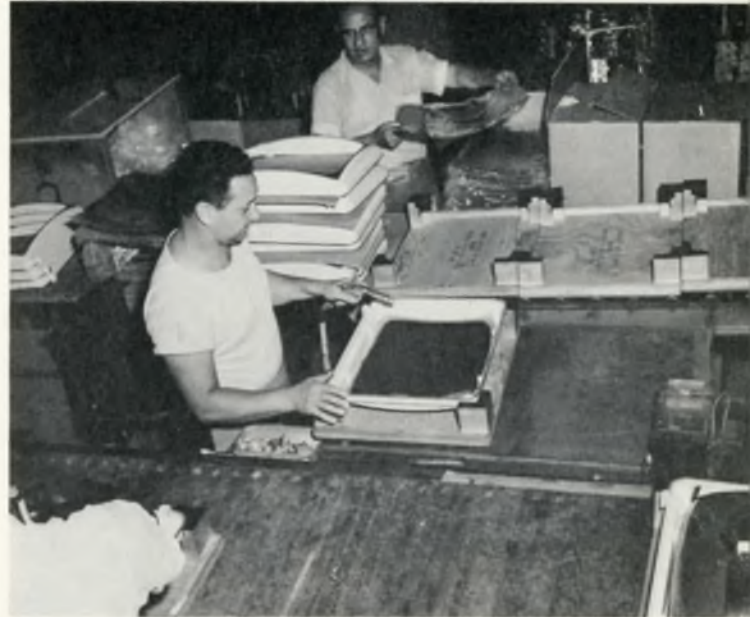
ANGELO SALVATORE , Dep't. 43-503, using anti-static air gun suggested by award winner Leone Carapucci in the Television Production Plant. This suggestion keeps TV masks free of dust and lint, and thus helps Philca remain "Famous for Quality the World Over."
