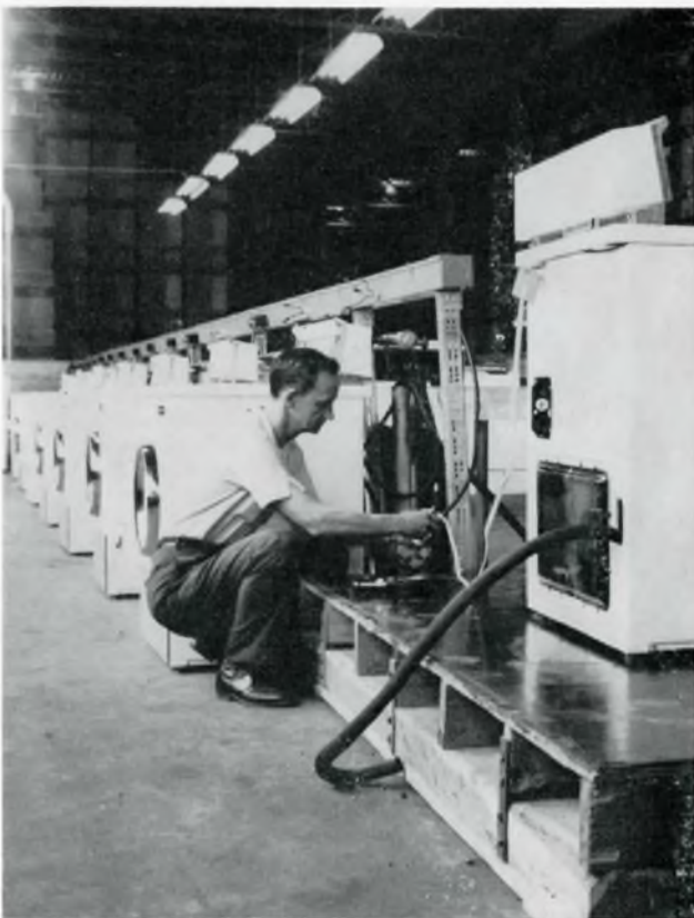
LIFE TEST installations are meant to duplicate those expected in homes. Washer mounted on section of conventional floor may reveal fault that would not show up if it were set on concrete.
