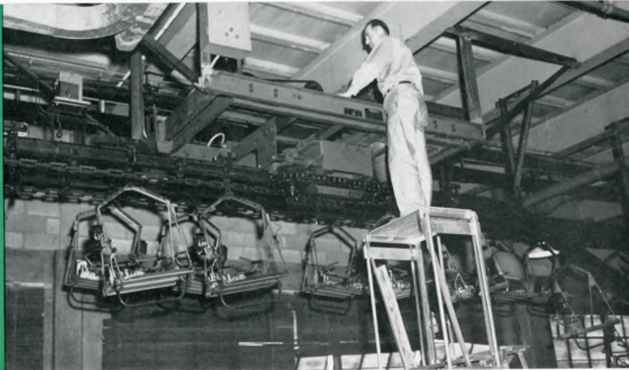
ED WILEY ADJUSTS a balanced monorail drive for the heat run conveyor which is so important in insuring Philco quality.
