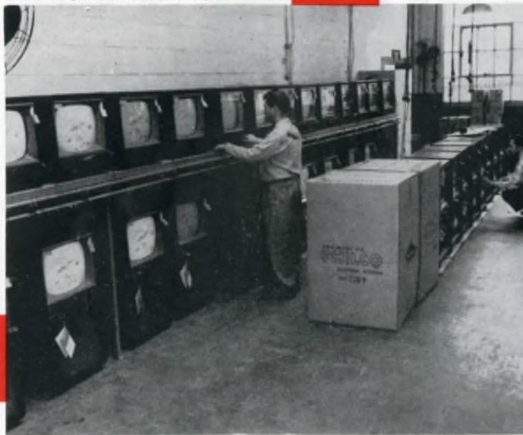
4. Packed stock sets of the first production are rushed to Plant 16 for thorough checking and 40-hour performance tests before the model is released for shipping. This is final proof that the quality and performance of the production receivers are up to the original standards set up for the particular model. ▼
