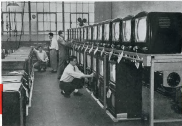
5. Daily thereafter, random packed stock is shipped to Plant 16 and these same tests are continued to see that our quality and performance have not "slipped" from the high standards. ▼
