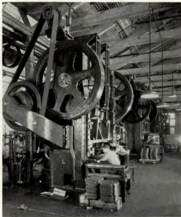
Fig. 2. Giant Double Crank Punch Presses, exerting 350 tons pressure, forming a sub-base for Philco Radio Chassis
