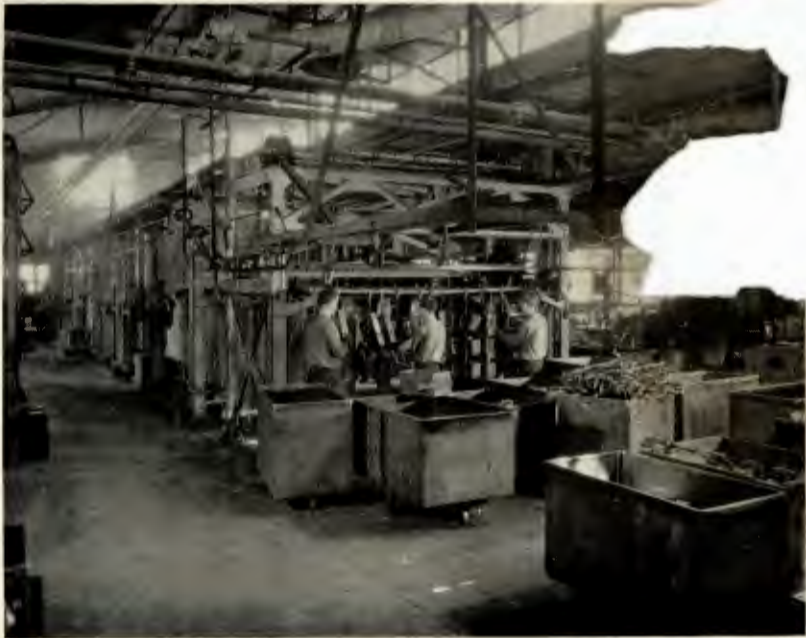
Fig. 3. Automatic Cadmium Plating Machine, 83 feet in length. All metal parts are cadmium plated to make them rust proof
