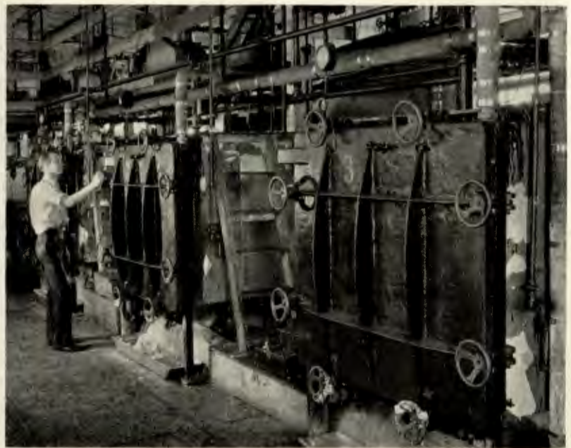
Fig. 6. Combination Vacuum and Wax Impregnating Ovens. This treatment makes Philco condensers absolutely moisture proof and trouble free
