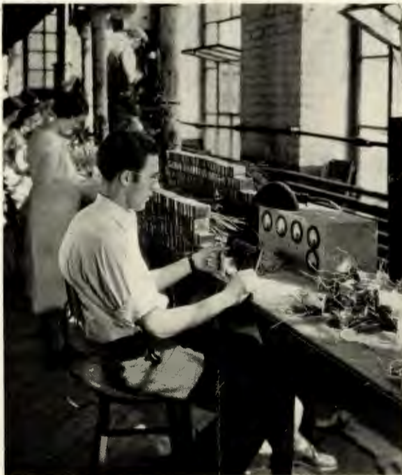
Fig. 7. Philco inspector testing completed By-Pass Condensers
