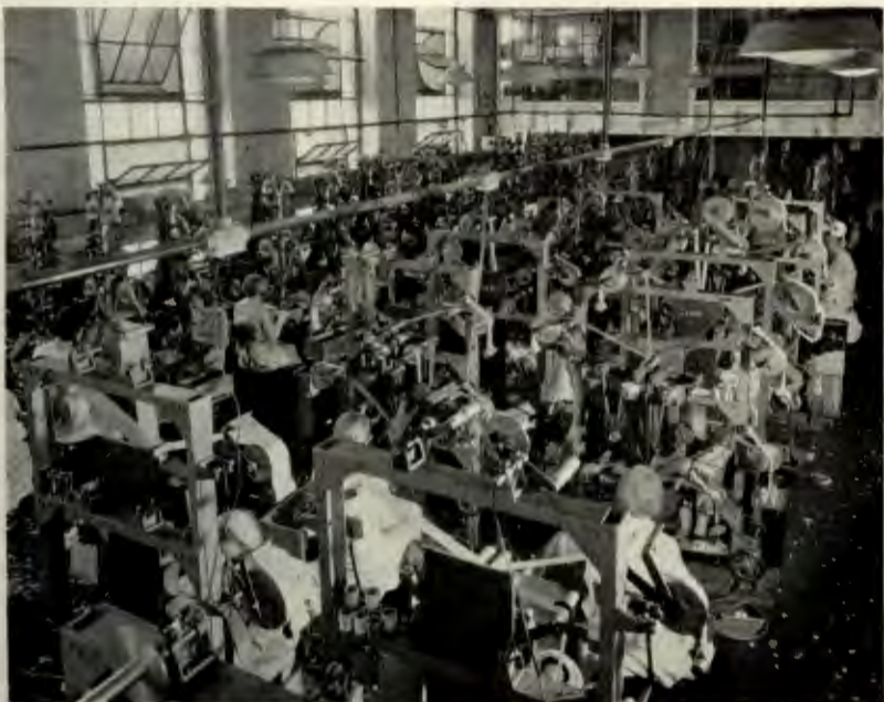
Fig. 5. The maze of Condenser Winding Machines, operating in a special room of never-changing humidity
