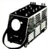
3 inch TV Oscilloscope Model S-8200. The most versatile and available in the field service. Probe built-in. Fast sweep. Sweep rate from 10 to 100 MHz. Also used for testing of high sensitivity TV receivers.
