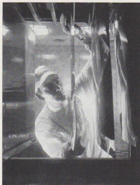
Shadowmask sheets after coating with photo-sensitive etchant resist.
