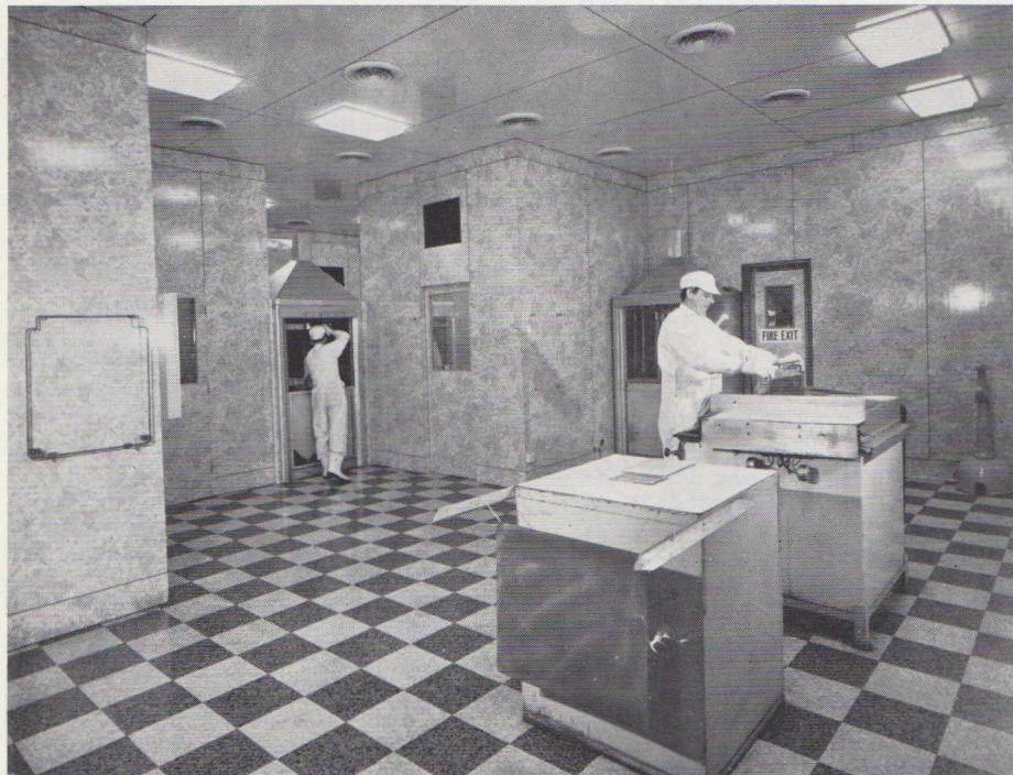
General view of developing area for shadowmask sheets where sensitised sheets are "developed" after exposure to ultra-violet light: the emphasis on dust-free conditions is apparent.
