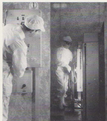
A shadowmask sheet is exposed to ultra-violet light.
